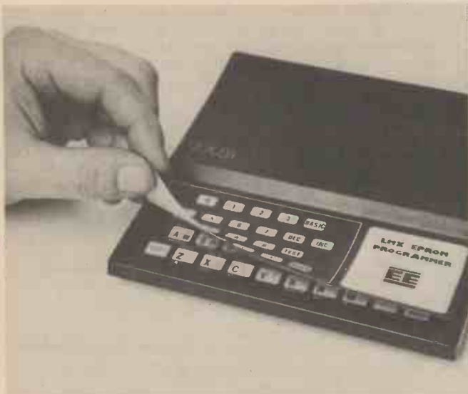
The keyboard overlay is held secure using double-sided tape at the top corners.
