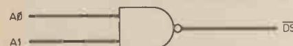
Fig. 8.3. 2-input NAND gate symbol and truth table. Device select low when 2-bit address 11 appears.
