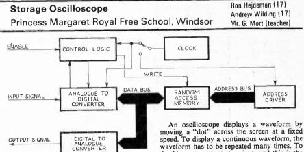
There is a type of oscilloscope which can do this, known as a storage oscilloscope, however, these are expensive, therefore an unviable proposition for schools. As a result, an alternative was designed to convert a normal oscilloscope into a storage instrument.
