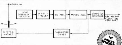
resistor placed just above the electromagnet is obtained by the pendulum preventing light falling on it. This pulse is then fed into a bistable, which causes the bistable to change state and remain so, until a second pulse is supplied. As soon as the bistable has changed state a pulse is supplied to a monostable causing it to change state. The output from the monostable causes a large current to flow in two transistors wired as a Darlington pair.
