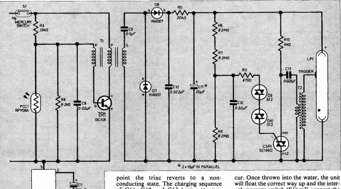
point the triac reverts to a nonconducting state. The charging sequence of C11, C12 and C13 begins to commence once more, and the cycle of events described repeats continuously until the power source is removed.
