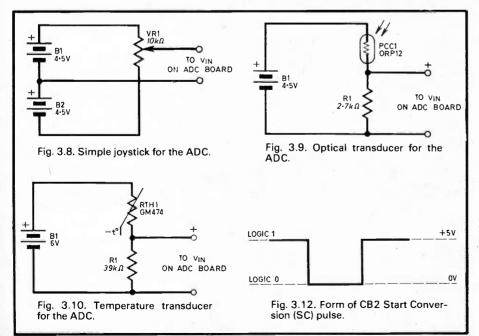
The start conversion (SC) pulse, necessary to initiate the conversion process, can be obtained in a variety of ways but it is often appropriate to put the ADC entirely under microprocessor control and derive the pulse from an output line available at the microcomputer. The shape of the pulse necessary to start conversion for the ZN449 is illustrated in Fig. 3.12.
