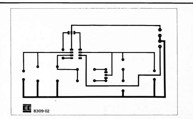
Fig. 3.15. Master pattern (actual size) to be etched for the Signal Conditioning Amplifier. This board is available through the *EE PCB Service*, Order code 8309-02.
