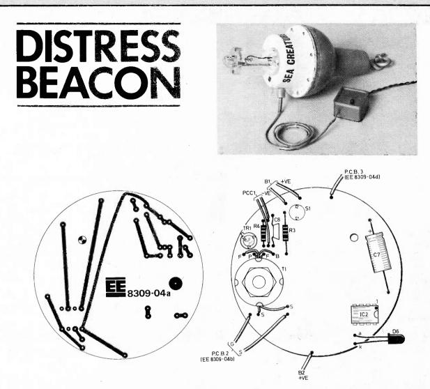
Fig. 2. The component layout and full-size artwork of p.c.b.1. Note that D6 is mounted at the top of the Beacon housing. Battery B2 is located on the space in the centre of this board.
