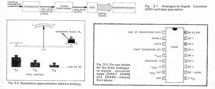
which hence determines the overall conversion time. A complete conversion occupies nine clock cycles so, for example, a ZN448 running at a clock frequency of 900kHz will give a conversion time of  $10\mu s$  and therefore a conversion rate of  $100,000s^{-1}$ .
