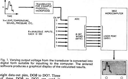
of these  $DO\emptyset$  to DO2 are used in selecting the required channel with DO3providing the necessary decoded  $\overline{CS}$ . The other four data-out lines are available to the user at SK9 to SK12 so that the computer may be used to control other equipment such as motors that may be required in A-to-D experiments for such purposes as transducer position and movement.
