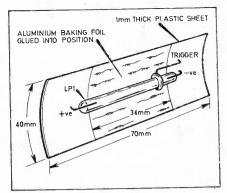
Fig. 10. Constructional details of the xenon tube reflector. The tube supports should be formed from well insulated, stiff wire.
