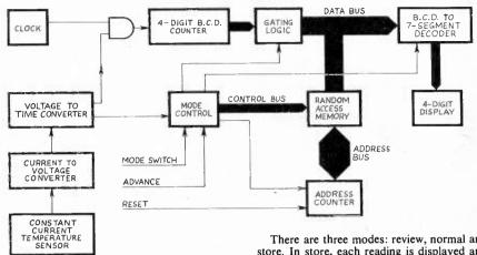
These are counted by a 4-digit b.c.d. counter. The control logic, routes each reading to and from the memory, display and counter via a data bus.
