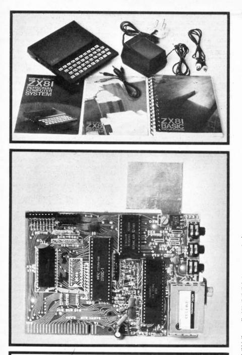
(Top) The ZX81 package comes with computer, 9V power pack (excluding mains plug), programming manual and leads for TV and cassette. (Above) The p.c.b. showing the finger set to connect the printer and extra memory.
