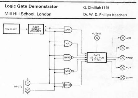
The circuit design consists of a multivibrator producing pulses at approximately 1Hz. These pulses are then fed to a 2-bit binary counter which drives the inputs of the five logic gates. The output to be displayed is selected by means of the gate selector switch and at the same time the corresponding indicator lamp is illuminated.
