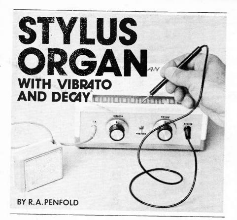
T HE Stylus Organ is basically a conventional instrument which covers two octaves (including sharps or flats), one octave either side of middle C. It has a switchable vibrato oscillator, the use of which gives a more "rich" and pleasant sound. An unusual feature which can further enhance the sound, is a simple envelope generator circuit, and this gives a fast attack time with a decay time which can be varied from a fraction of a second to several seconds.
