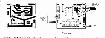
Fig. 5. The full-size artwork and component layout of the battery charger p.c.b. This fits into a small enclosure into which D2 is mounted.
