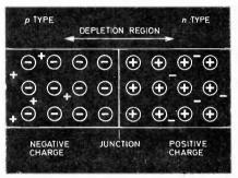
Fig. 5.5. A *pn* semiconductor junction. The charges shown encircled are fixed in position by chemical bonds, whilst the others are free to move.
