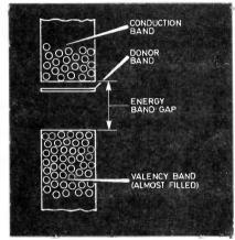
Fig. 5.2. Energy band diagram of an *n*-type semiconductor material.
