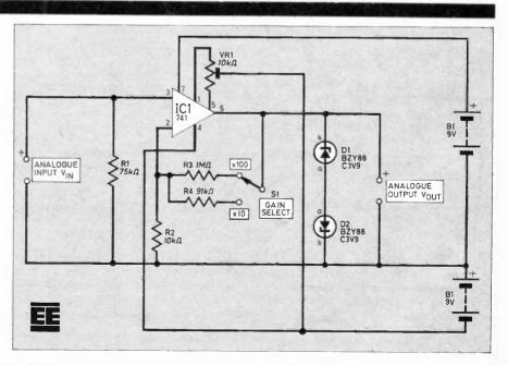
Fig. 3.14. The circuit diagram of a Signal Conditioning Amplifier for use with the ADC.
