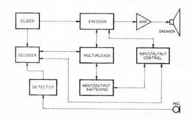
speed of data transmission, this meant an accurate clock was needed. The accurate clock pulse is provided by a crystal oscillator.
