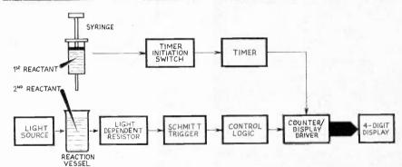
The timer itself consists of a light shining through the reaction vessel onto a light dependent resistor (l.d.r.). As the precipitate thickens the resistance of the l.d.r. increases and this increase is used to control a switching circuit, which in turn stops a 4-decade counter timing the reaction.
