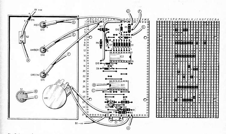
Fig. 2. Layout of components on the topside of the stripboard and interwiring to the front panel of the case. The underside of the board detailing breaks in the copper strips is shown far right.
