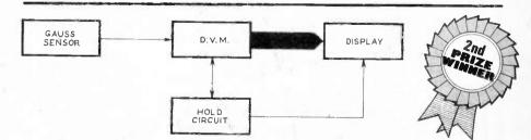
ted in a probe. The sensor gives a differential output, dependent on the strength and polarity of the magnetic field. This is fed into a digital voltmeter i.e. The sensor is biased to be linear up to  $\pm 3000$  gauss.
