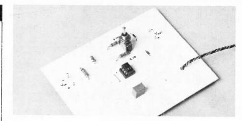
The power supply for the circuit needs to be a split type ranging from  $\pm 6V$  to  $\pm 15V$ ;  $\pm 9V$  was selected as this is readily available in battery form. Two PP9 batteries will give long service.
