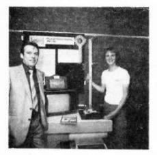
THE object of this project is to determine a value for "g", the acceleration due to gravity, using a pendulum linked to a BBC Microcomputer. Experimental time is reduced and a fairly accurate value of "g" may be determined. It can also be used to show how errors can be reduced by increasing the number of pendulum swings.
