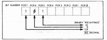
Fig. 3.13. The Peripheral Control Register (PCR) in pulse output mode. The three most significant bits control the mode of operation of the CB2 line.
