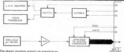
The design revolves around an analogue-todigital converter which converts the varying analogue voltage from a normal pH meter and digitises it, so that it can be used by the 380Z. Before this stage there is a variable gain amplifier and buffer which obtains full graphical range from the 380Z.
