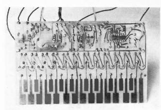
The track-side of the p.c.b. showing the keyboard area. This is polished but not coated as good electrical contact is required with the probe tip.
