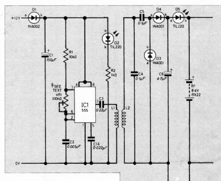
Fig. 1. The circuit diagram of the marine version of the Distress Beacon. The circuit for the pocket version (see Figs. 9, 10 and 11) is identical with the exception of the battery charger section (to the left of B1 and B2) and PCC1, which are omitted.
