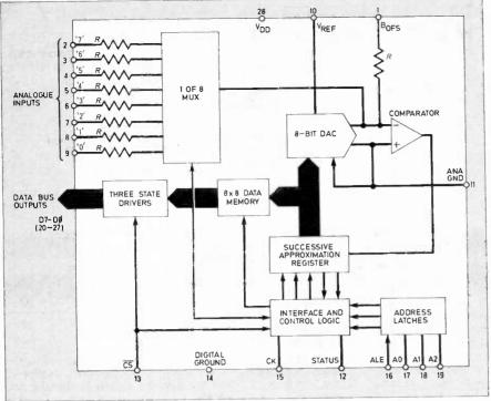
Fig. 3. Internal block diagram of the 7581 A-to-D converter i.c.
