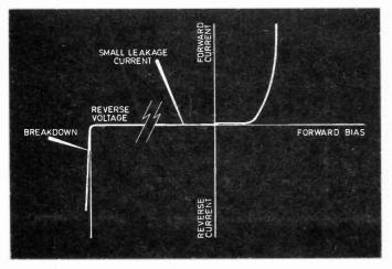
There is therefore a region on each side of the junction which is depleted of charge carriers; this is known as the depletion region.
