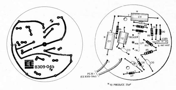
Fig. 3. The component layout and full-size artwork of p.c.b.2. The xenon tube, LP1, is mounted onto stiff wire supports in the holes indicated (see also Fig. 4).
