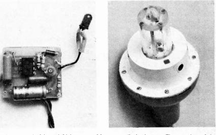
The charger p.c.b. (above left) is mounted into a small plastic case. The top view of the Distress Beacon (above right) shows the light dependent resistor and the recepticle for the charger coil. Below, the shape of the charger coil can be seen.
