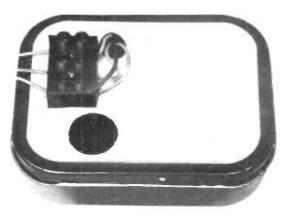
The completed unit with a 3-way terminal strip fixed to the lid of the case.
