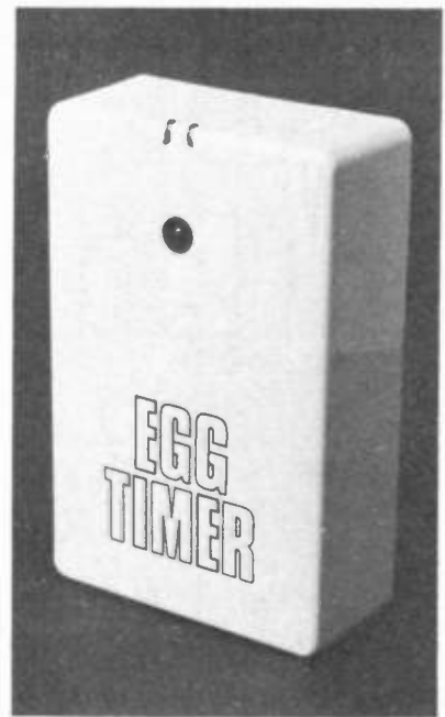
Photographs showing the unit with the case lid removed, and right, the finished Egg Timer with the touch contacts on the top corner.
