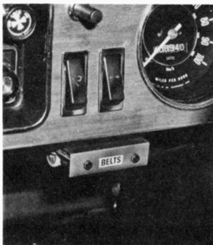
The Seat Belt Reminder mounted beneath the dashboard of the authors car, where it can be seen by both driver and passenger but is not too obtrusive.
