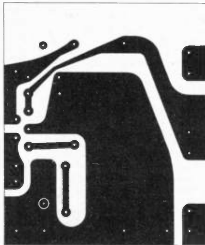
Fig. 3. The full-size master pattern to be etched on the p.c.b. The black areas represent the copper tracks.
