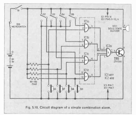
The combination alarm of Fig. 5.10, can be used as the basis of many kinds of combination lock circuits. Here it is used to sound the alarm when a person not in the know opens the door of a room or cupboard. S1 is the master switch, hidden just inside the doorway. S10 is a microswitch, open when the door is closed. but closing whenever the door is opened. S2 to S5 are switches inside
