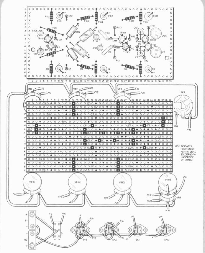
Fig. 2. The circuit board of the 3-channel Stereo Mixer. (Top) topside of board showing all components in situ. (Below) strip-side of board showing all breaks in copper strips. Also, note that the interconnecting leads are soldered to the strips as indicated by the solder "blobs".
