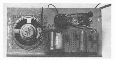
View of the rear of the front panel showing circuit board in position.
