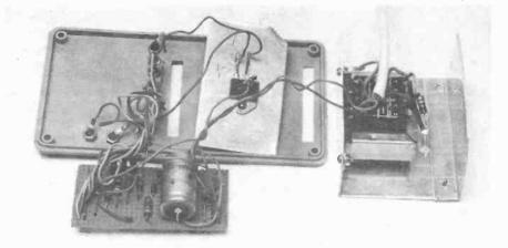
Exploded view of interior components of the battery charger. The transformer mounted on its heat sink can be seen on the right with the transistor laying on top of the front panel in the centre of the picture. The circuit board is lying below the front panel.
