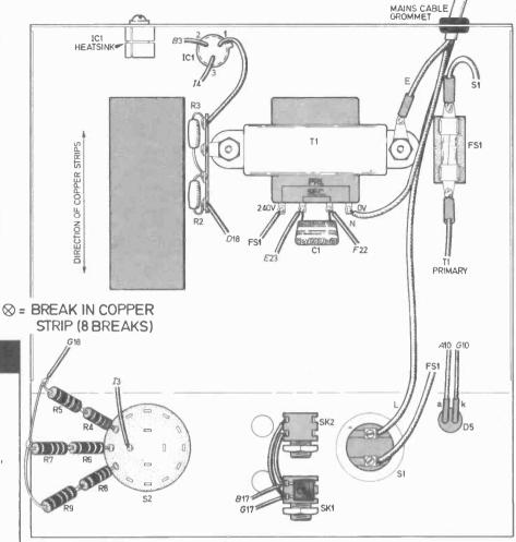
Fig. 2. Circuit board layout and interconnection diagram. The heatsink for IC1 must be insulated from the metal chassis.
