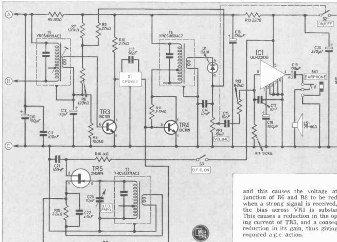
Fig. 3. The remainder of the circuit diagram containing the r.f. amplifier, detector, a.g.c., audio and b.f.o. stages of the 4-Band Radio.
