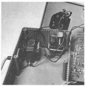
Position and wiring of transformer and relay fitted in the case.
