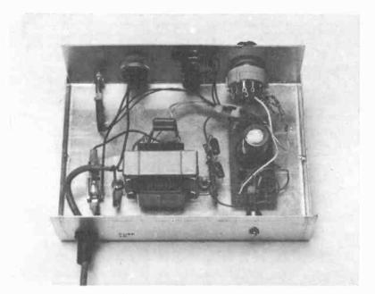
Interior view of the unit from the rear. The wiring to the front panel mounted controls can be clearly seen.
