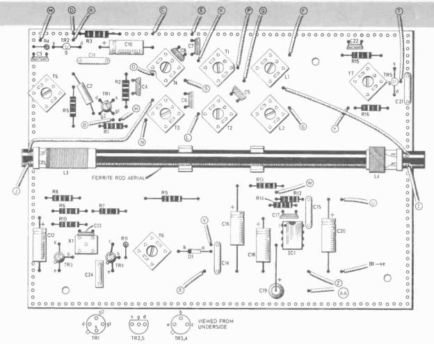
Fig. 4. The layout of the components on the topside of the circuit board and their interconnection (below) on the underside. Also shows flying leads to the case mounting components.
