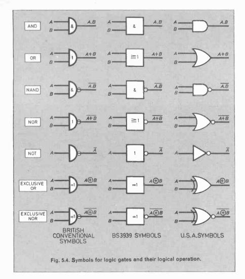
inverse of the output of an AND circuit (Fig. 5.1b). The output is INVERTAND OF NOT-AND, usually shortened to NAND.
