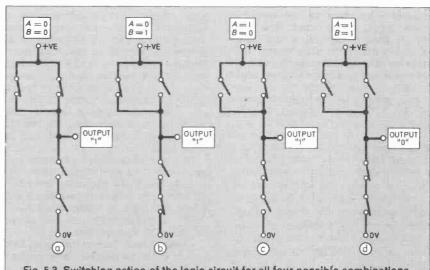
Fig. 5.3. Switching action of the logic circuit for all four possible combinations of input conditions. "0" = 0V and "1" =  $\pm$ 9V.
