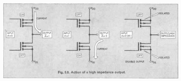
buses, but can be in effect disconnected under electronic control whenever necessary. When one i.c. is connected to the bus and transmitting data signals, the outputs of all other i.c.s wired to that bus are in the high impedance state so that they act as if they were not really there.
