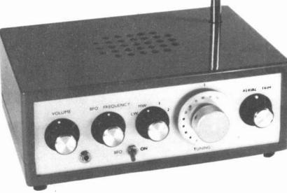
A PART from covering the standard medium and long wavebands, this receiver additionally has two short wave ranges covering from about 1.6MHz to 4.5MHz, and 4.6MHz to 14.6MHz.
