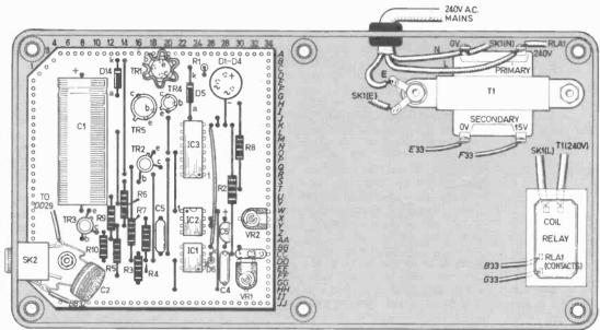
RELAY SOCKET MOUNTED ON 'L'SHAPED BRACKET
