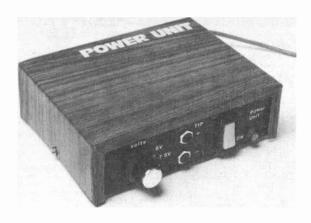
Exterior view of the completed power supply showing front panel controls and labelling.
