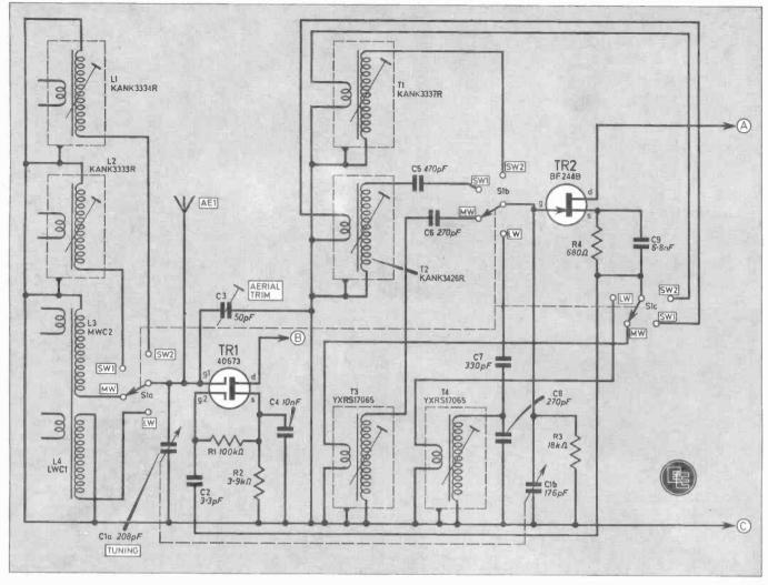
Fig. 2. The circuit diagram of the mixer and oscillator section of the 4-Band Radio.
