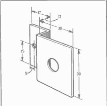
Fig. 6. Drilling and bending details of the tuning capacitor brackets.
