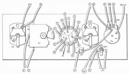
Fig. 5. The layout and interwiring of the front panel mounted components. See photograph and text for C3/C1 bracket fixing details.
