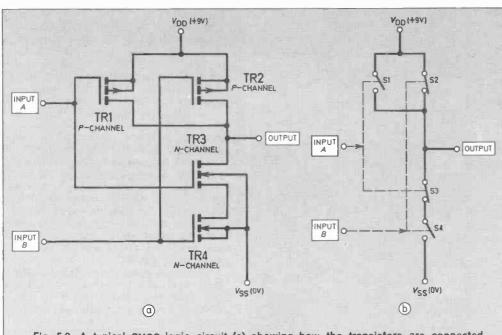
Fig. 5.2. A typical CMOS logic circuit (a) showing how the transistors are connected (b) equivalent circuit employing pairs of switches.
