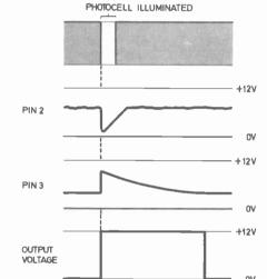
Fig. 2. Voltage changes occurring at ICI input and output when the photocell is illuminated.
