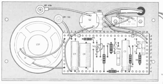
Fig. 2. Circuit board layout and component interwiring. Note that several components are mounted in the probe. Connections to the probe are made via twintcore screened cable to minimise signal loss. Conductor a in the probe corresponds to wire a at \$1, and similarly with conductor b.
