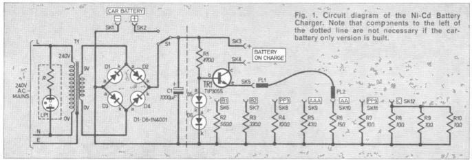
For quite a wide variation in operating conditions, therefore, the charging current will be fairly constant. This state will be maintained so long as no more than approximately 9 volts of batteries are connected to the output.
