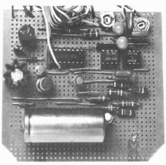
The completed prototype circuit board. Here C6 is constructed from two  $47\mu$ F capacitors wired in parallel.
