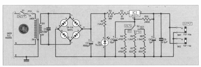
Fig. 1. Full circuit diagram of the Uniboard Power Supply.
