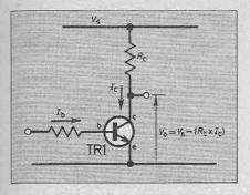
Fig. 8.3. A simple transistor switch using the common emitter configuration. The base current must be greater than that just needed to saturate the transistor.
