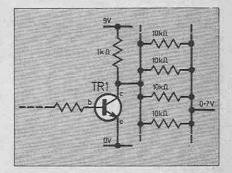
Fig. 8.5. The loading on the switch in Fig. 8.4 can be redrawn thus. The load appears as a number of  $10k\Omega$  resistors in parallel all to 0.7V.
