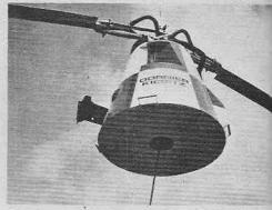
Spy in the sky. A German Dornier "Kiebitz" tethered rotor platform goes aloft from its support truck. Unmanned, it takes electronic equipment up to 1,000ft greatly increasing its operation range.
