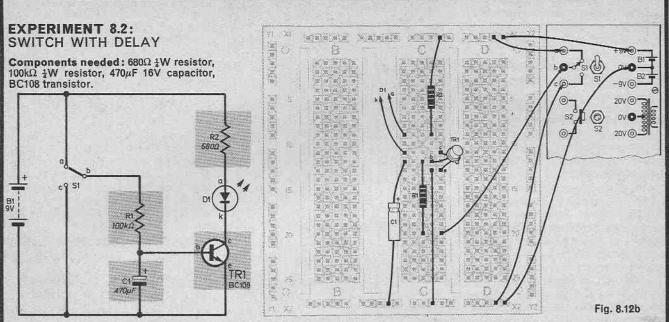
Fig. 8.12(a) Circuit diagram of Experiment 8.2. (b) Layout of the components on the Tutor Deck for Experiment 8.2.
