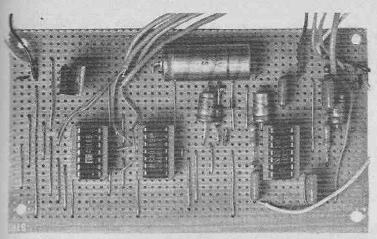
Layout of components on the completed circuit board for the Auto Fade. We strongly recommend the use of i.c. sockets as the i.c.s can easily be damaged during soldering.
