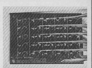
The left hand photograph shows a view of the top of the lockout board. Note the use of ribbon cable for off-board connections. The other photo shows a view of the modelling network board. Note the circular shaped plastic encapsulated BC108 transistors and copper bus wires.
