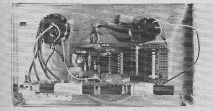
The fully wired chassis assembly with aerial secured to board.
