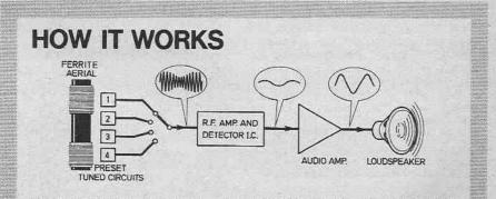
Radio frequency signals from the transmitter induce voltages in the coils on the ferrite rod aerial. Four r.f. tuned circuits are formed with the aerial which can each be inputted to the r.f. amplifier/detector i.c. The output from this is the required audio signal which receives boost from the audio amplifier to be heard in the loudspeaker.
