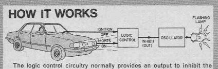
The logic control circuitry normally provides an output to inhibit the operation of the oscillator (it does not oscillate). However, when a condition arises where the lights are on and the ignition is turned off, the logic output changes and allows the oscillator to operate. This activates a warning lamp (or buzzer) inside the car to flash (or sound). The logic circuitry has a built-in parking facility which is enabled by turning the lights off and then on after the alarm has sounded.
