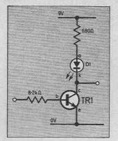
Fig. 8.7. If it is desired to drive a light emitting diode from one of our switches then the circuit shown can be used.
