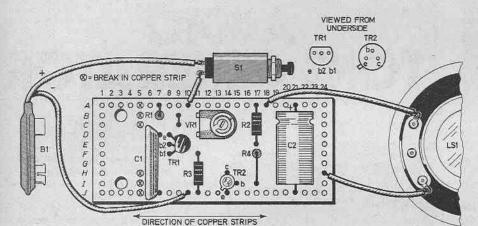
(above) The completed circuit board, The use of a heatsink for TR2 is optional.
