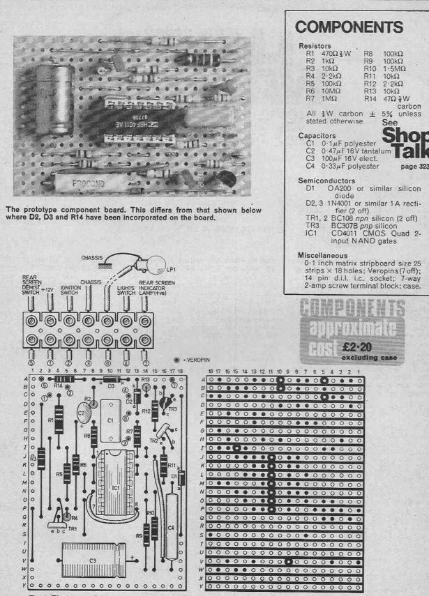
Fig. 2. The layout of the components on the topside of the board and the breaks to be made in the copper strips. Numbered leads from the terminal block refer to Veropins on board. Only one indicator lamp should be used, either LP1 or existing panel lamp for some other function (e.g. rear screen demister indicator).
