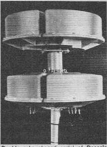
Double cake shaped aerial of Decca's EW equipment. Being designed to fit around a mast, it does not compete for the sought after masthead position.
