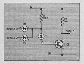
Fig. 8.9. The circuit shown is a logical NAND gate. Only when both inputs are high does the output go low.
