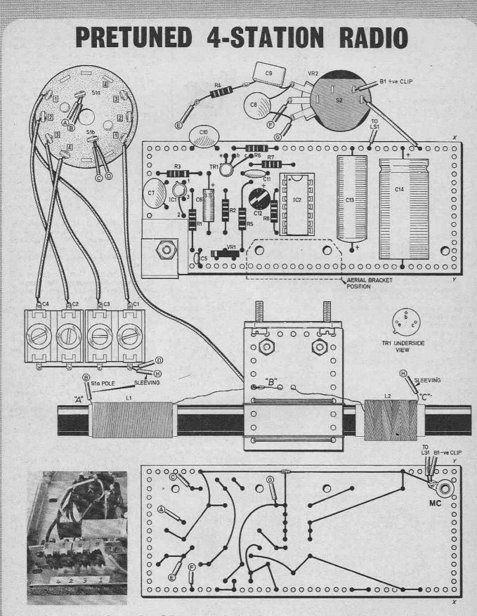
A close-up view of the trimmer capacitor bank showing fixing brackets used in the prototype. Fig. 2. Full construction details showing the board and components in their relative positions in the case. The L-shaped aerial bracket is bolted to the circuit board. The trimmer capacitor brackets will need to be constructed to suit the trimmers obtained. One bracket is fitted by one of the board fixing bolts with the other on the chassis. However, this may need alteration.
