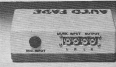
Rear view of the unit showing the phono socket strip and mic. input jack socket.
