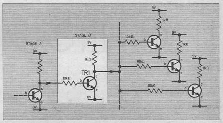
Fig. 8.4. The transistor switch (Fig. 8.3) as it looks when in a system. Note that only one output feeds it whilst it feeds many inputs.
