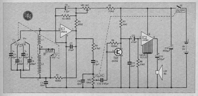
Fig. 1. The full circuit diagram for the Pretuned 4-Station Radio. The coils with ferrite rod core is a standard ready made component type FR5.
