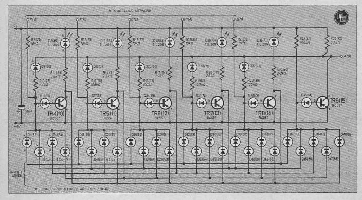
Fig.4. Complete diagram of the lockout circuits. Note that two of these are required, one for the rows and one for the columns. Bracketed component references are for the column lockout circuit and unbracketed ones for the row lockout circuit. These are both built on board B.
