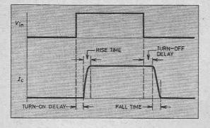
Fig. 8.6. When a pulse is applied to the input of our switch the output does not change instantly but with the delays as shown here.
