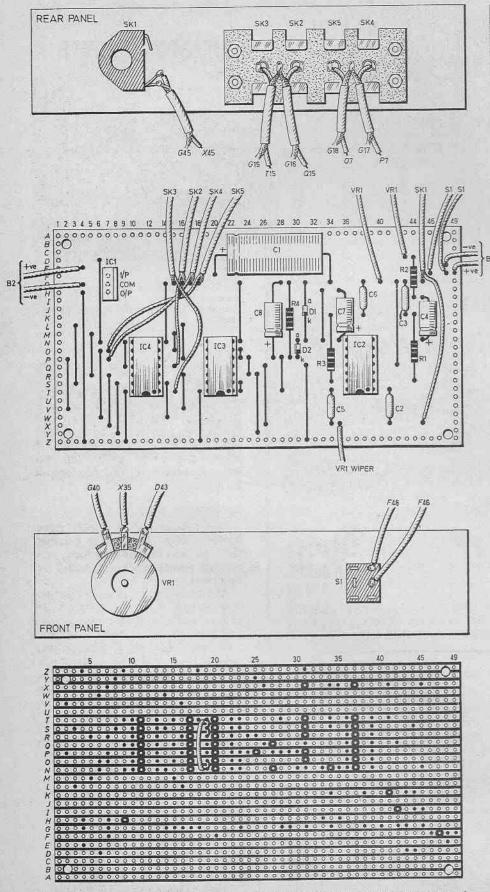
Fig. 2. Complete wiring details for the Auto Fade Unit. Be extra careful when wiring the links, as a mistake will be difficult to trace later on. Note the four links on underside.
