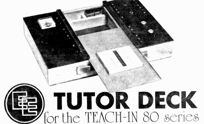
In order to follow the experiments in the Teach-In 80 series, it is recommended that the experimental Tutor Deck described here is constructed. The following instructions describe the construction of the deck referred to in the series but the design can be adapted to suit requirements of the user.
