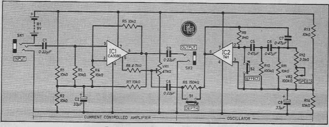
Fig. 2. The complete circuit diagram of the Tremolo Unit.
