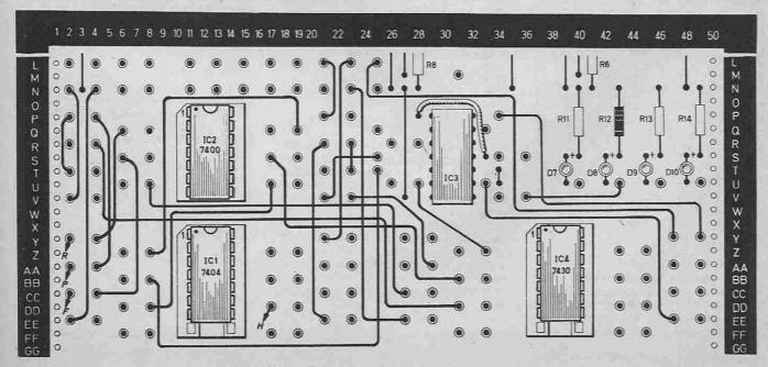
Fig. 9.2b. The circuit of Fig. 9.2a built up on the Test-Bed.
