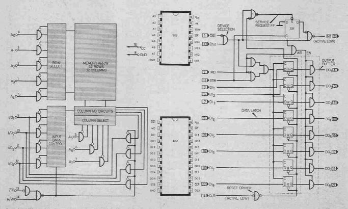
Fig. 4.1. The Intel 2112 1,024-bit Static Random Access Memory. No "refreshing" is required with this type of RAM.
