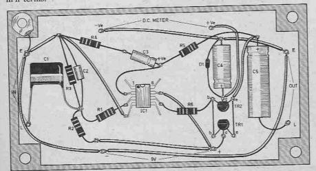
Fig. 2. Plywood circuit board glued to Formica front panel. All components and wiring soldered to miniature household pins.
