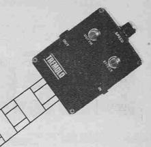
The input impedance of the circuit is approximately 8 kilohms which should suit most electric guitars.
