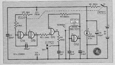
Fig. 2. Complete circuit diagram of the Metal Locator.
