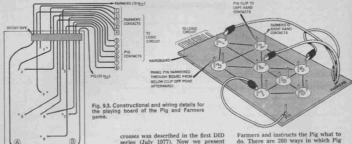
There are five NAND gates each corresponding to one of the statements, and each fed by two inputs either direct or inverted.
