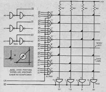
Fig. 4.4. Circuit for the homebrew ROM, made up from standard TTL components.
