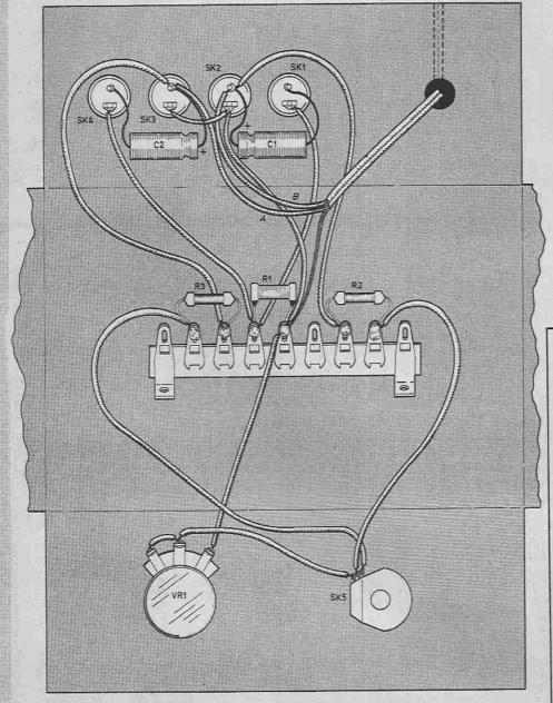
Fig. 4. Complete wiring details for the unit. Note the case has been "opened out" for clarity. There is nothing critical about the layout and could be varied as required.
