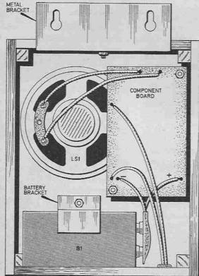
Fig. 3. Final interwiring details, showing the relative positions of the components. If a ready made case is used then a slight change in positioning may be necessary.
