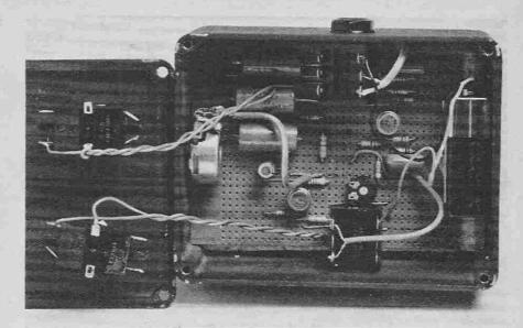
The completed prototype unit with lid removed showing case mounted components, board positioning and wiring to the lid mounted switches.
