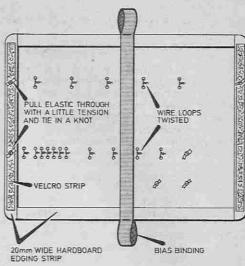
Fig. 4.1. Construction details for the tool board. The elastic retaining strips are partioned and anchored by means of twisted insulated wire. Use of Velcro enables easy removal of the board. The component boxes are glued to the baize.
