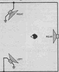
Fig. 1. Hafler's basic idea of adding a single speaker.
