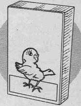
THE TWITTERING OF Chirping sound from this Electronic Canary unit is very distinctive, and will find use in replacing the traditional door bell or buzzer. Children will also find the sound novel, and will doubtless play with it purely for fun. Operation is economical, the current drain from a PP6 battery being very low and will give many hours of use.
