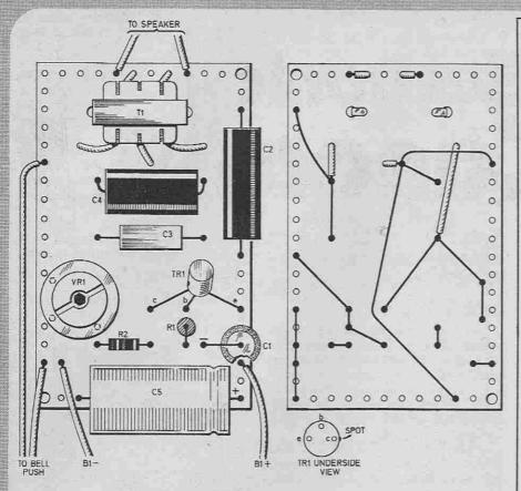
Fig. 2. Matrix board layout. The style of the preset may differ from that shown, but the connections will remain the same.
