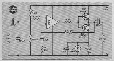
use a new value for R4, calculated from: R4 (new=100 kilohms (A-1) where A is the required gain.
