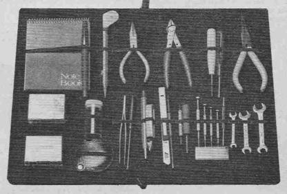
The prototype tool board removed from the lid of the briefcase for use on the construction bench.
