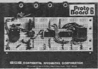
PB.6 Kit, 630 contacts, four 5-way binding posts accepts up to six 14-pin Dips.
