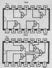
Fig. 9.5. Pinning details for the 7408 and 7454 logic i.c.s.
