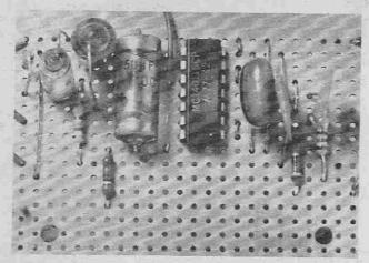
Layout of components on the completed circuit board for the Low Cost Metal Locator.
