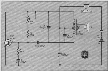
Fig. 1. Complete circuit diagram of the Electronic Canary.
