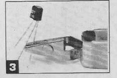
Quite a selection of transistor types are used in constructional projects in EE, but in most cases each can be changed for other type numbers you may have in stock that have similar electrical characteristics, without affecting circuit operation. They may even have different pin-out arrangements and case styles, but the leads can easily be re-formed to suit.
