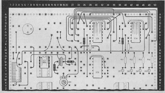
Fig. 8.3(b). The circuit of Fig. 8.3(a) wired up on the Test-Bed; S4 must be switched on.
