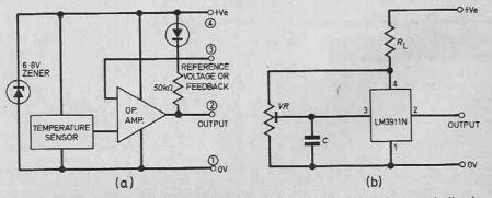
Fig. 1a. Block diagram of the circuit inside the LM3911N temperature controller i.c. (b) Illustrating the method of using the i.c. as a switching type thermostat.
