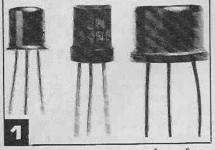
made from Transistors are "treated" wafers (or chips) of silicon or germanium-the latter being used less and less due to inferior performance compared to silicon devices.
