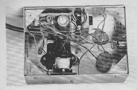
strips. Next the various components and the single link wire are soldered into position on the board, and the two  $3 \cdot 2mm$ diameter mounting holes are drilled in the board. The point to point wiring must then be completed before the component panel is mounted next to T1 on the rear of the case.
