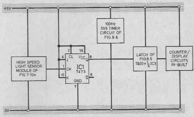
Fig. 8.5. Block diagram of a light triggered timer.
