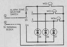
Fig. 5. Circuit for choice of remote alarm.
