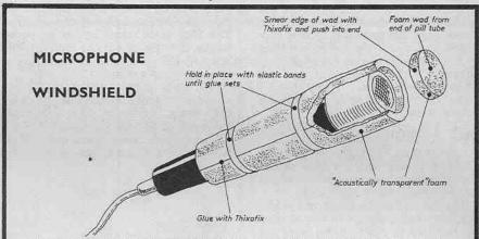
Fig. 1. Construction of the Microphone Windshield. It is important to make sure you use only a thin coating of glue to avoid sticking the foam to mic case.
