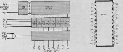
Fig. 3.2. The Signetics (Mullard) 82S190 16K Programmable ROM. An example of a fusible-link device, for field programming.
