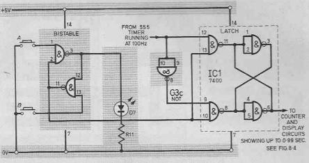
Fig. 8.4. Circuit diagram of a reaction timer.
