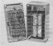
Board mounted on the lid of the case and housing of the batteries.
