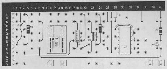
Eventually the charge reaches two thirds of  $V_{\rm CC}$ ; circuitry connected to pin 6 detects that the value  $2/3V_{\rm CC}$  has been reached, causes output to go low again, and begins the rapid discharge of C1 through pin 7.
