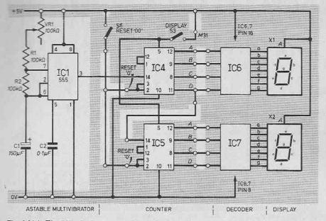
Fig. 8.3(a). The 555 wired as an astable multivibrator in an event timer up to 99 minutes in steps of one minute.
