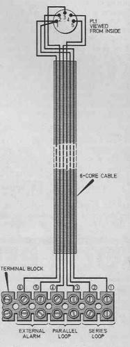
Fig. 4. Wiring up a terminal block to a 5-pin DIN socket.
