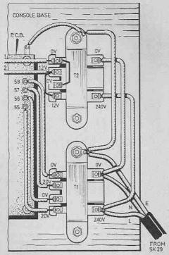
Fig. 3.3. Shows position of the transformer alongside the p.c.b. and wiring details. Note the use of solder tags for earthing purposes, particularly the one at the p.c.b. fixing. This must be in good contact with the earth plane on the board underside.
