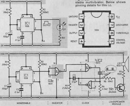
Fig. 8.2(a). An audible alarm is produced at a preset time after grounding point A.
