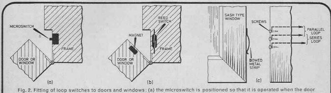
Fig. 2. Fitting of loop switches to doors and windows: (a) the microswitch is positioned so that it is operated when the door opens/closes; (b) using a reed switch and magnet. When the door closes the magnet causes the switch to close (suitable for series loop); (c) a home-made switch constructed from brass plate and screws. A dual type is shown for connection in both parallel and series loops.
