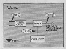
Fig. 1. Block diagram showing the various stages of the converter and the principle of operation.
