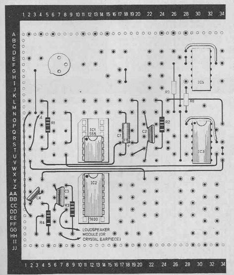
Fig. 8.1(b). The circuit of Fig. 8.1.(a) wired up on the Test-Bed. Try different combinations of values for C1 and R1 and observe the high pulse length.
