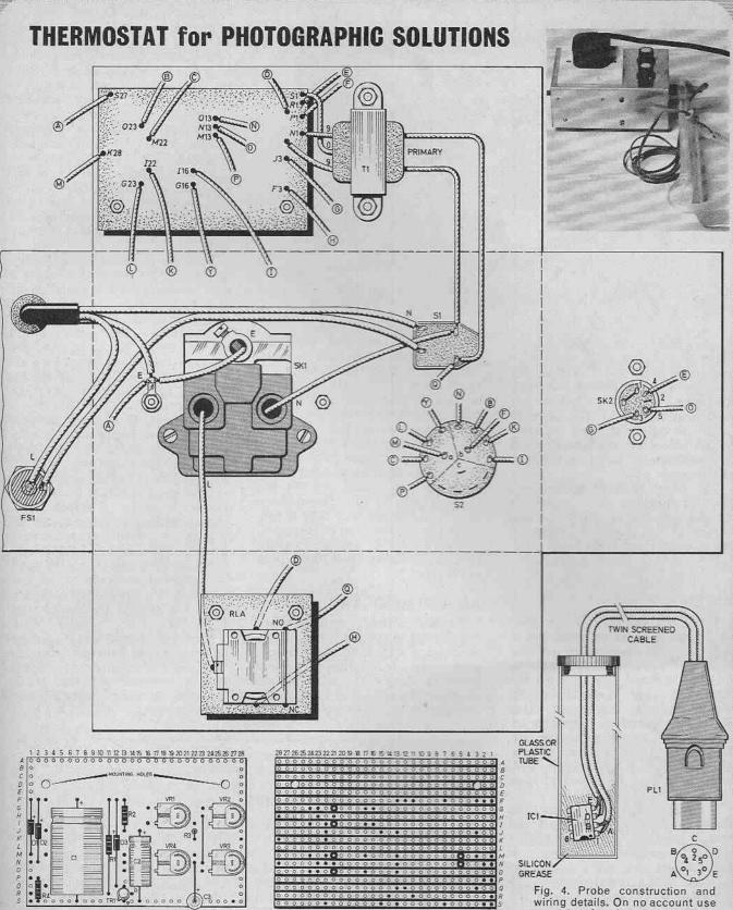
Fig. 3. Complete wiring details for the unit, showing the stripboard layout and other wiring. There is nothing critical about the layout and could be varied as required. When wiring up the mains socket, use mains rated connecting wire and insure that all connections are well insulated. The probe socket, SK2 needs particular care when wiring otherwise an incorrect connection will damage the i.c. The socket is shown looking at the tags. Note the earth tag connection.
