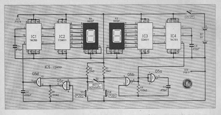
Fig. 1. The complete circuit diagram of the Electronic Dice.
