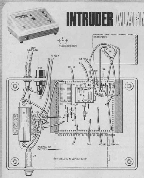
Fig. 3. Layout of the components on the stripboard and wiring-up details. Below shows positions of top-panel controls and wiring information. Note that the copper strip on the board underside is to be broken at two points, C13 and C18.
