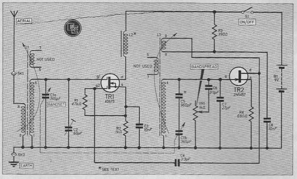
Fig. 2. Complete circuit diagram of the Short Wave Converter.
