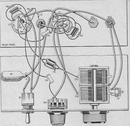
Fig. 4. Complete wiring details for the converter. Most of the components are mounted on the coils directly. When soldering TR1 be sure to leave the shorting clip in place, otherwise the device will be destroyed. Remember however, to remove it before switching on!
