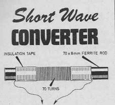
Fig. 3. Construction of the coupling coll L2. The coll is a single layer using 32 s.w.g. copper wire.
