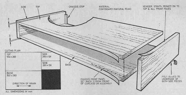
Fig. 6-1. A wooden case for housing the 2020 Tuner Amplifier.
