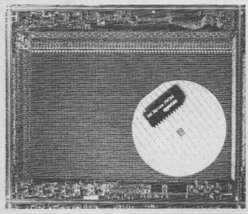
graph of the Signetics (Mulof the lard) 16K Programmable ROM (see Fig. 3.2) with inset photo's of one silicon slice which contains around 100 individual chips and an encapsulated chipthe final device.
