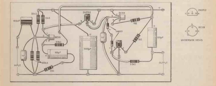
Fig. 8.10. Covercard required for the POWER AMPLIFIER. This is reproduced full size and may be traced directly.
