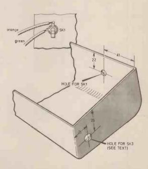
Fig. 8. Case drilling details. Locate p.c.b. assembly and check alignment of output socket SK2 before drilling hole for aerial lead connector.
