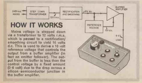
greater than that at the base by approximately 0.6 volts (base/ emitter voltage drop) producing an output voltage level of -9.4 volts (neglecting component tolerances).
