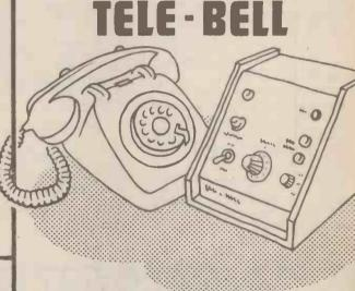
This sound-triggered device will let you know when your telephone is ringing if you are out of range of the in-built telephone bell, when working for example in the garden shed, garage or other remote location. Will find many other uses in and around the home.
