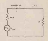
Fig. 8.4. For calculating the output current from an amplifier a simple equivalent circuit as here can be used.
