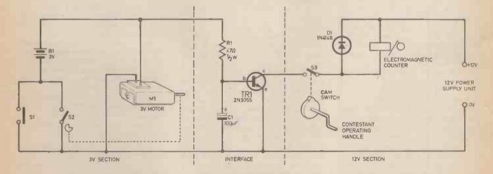
Fig. 3. Basic circuit of *The Thing* incorporating the various modifications The Prof. has been discussing. The resistance of the counter is not critical.
