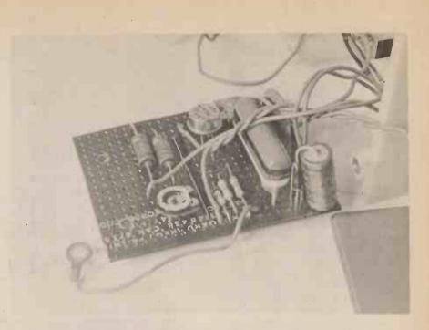
The Flashmeter circuit board removed from the case showing the layout of components.
