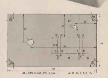
Fig. 7. Front Panel drilling details.
