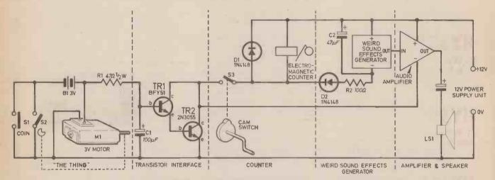
Fig. 4. Final circuit of *The Thing*. In this design all the extras have been included, namely the *Weird Sound Effects Generator*, and an amplifier.
