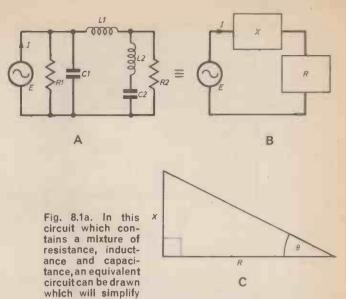
to just one reactance and one resistance as in (b). The cosine of a right angled triangle is represented as in (c).
