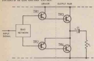
Fig. 8.8. If higher power is required from a complementary stage it is usual to use a circuit similar to that shown here. In this instance the circuit is called a quasi-complementary stage.
