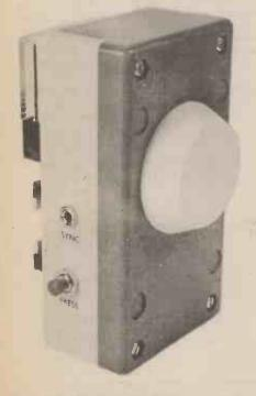
Rear of the finished unit showing the light diffuser.
