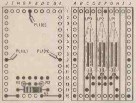
Fig. 2. Layout of components on the stripboard.
