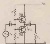
Fig. 8.7. A basic complementary output stage. Although both transistors should be identical with respect to their ratings, one should be npn and the other pnp.
