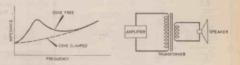
Fig. 1. Illustrating how the Impedance can vary with different positions of the speaker cone.
