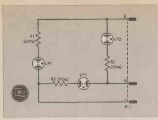
Fig. 4. The complete circuit diagram for the Mains Tester.
