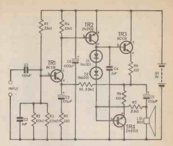
Fig. 8.9. The complete circuit for a practical amplifier. Again the circuit may look complicated but if thought about carefully can be broken down into sections guite easily.
