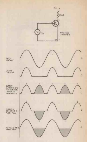
Fig. 8.5. A simple class B amplifier with an input waveform as shown will only produce the positive half cycles as in (b). If two similar transistors are used and their outputs added the waveform in (c) is produced. If however one of the outputs is inverted and added, the waveform shown in (d) will be the result. With a small bias a satisfactory output as in the last curve will be produced.
