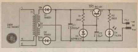
Fig. 2. The complete circuit diagram of the 9V d.c. Power Pack.
