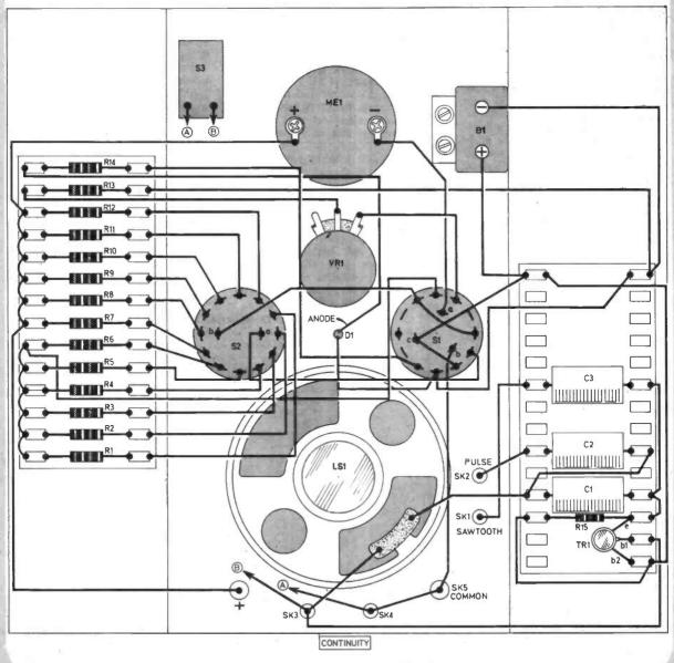
Fig. 2. Construction and wiring of the Multi-Tester.
