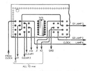
Fig. 4.4. Wiring of both flip-flops in the 7473.
