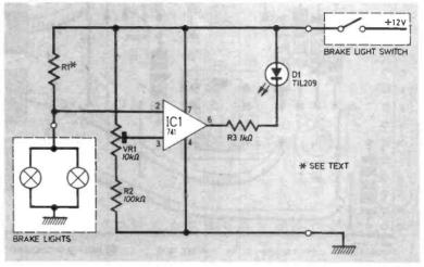
operational amplifier are derived from potential dividers across the supply lines. An adjustable reference voltage is produced by means of the divider action of R2 and VR1 in series. The input to pin 3 being taken from the wiper of VR1. The latter is used for limited fine adjustment. With VR1 set to midway position there is about 11.5 volts on pin 3.
