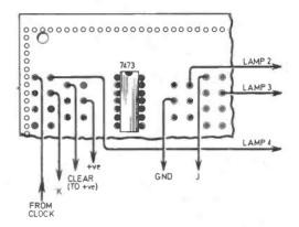
Fig. 4.3. Wiring of one flip-flop on the circuit board.
