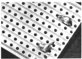
6 Two poor joints. In the upper one the solder has formed a blob on top of the copper and not run evenly over it. In the other the wire was not bent down, or cut short enough.
