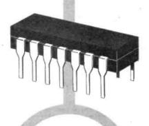
AVING LOOKED at integrated circuits containing simple two-input gates in previous parts of this series, we now go on to more complex integrated circuits, looking in particular at the dual J-K flip-flop i.c., type 7473.
