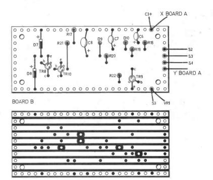
Fig. 4. Layout and wiring of the timer board.
