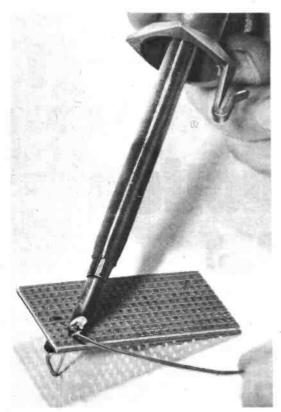
5 Making the joint. Melt a small amount of solder onto the joint, not onto the iron, wait just long enough for it to run evenly over the whole area then remove the iron.
