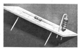
3 Two methods of component mounting on Veroboard. Bend the leads down in line with the strips and cut off leaving about 2 to 3mm.
