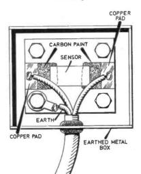
according to Fig. 1. It employs a piece of printed circuit board for mounting the sensor paper, with graphite conducting paint used to make the connections between copper and sensor, to avoid corrosion.
