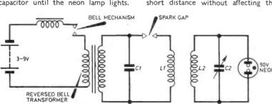
Fig. 1. The circuit of the spark equipment.
