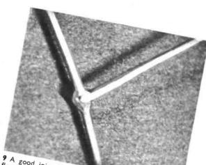
9 A good joint between two wires, the solder has the wires, and is clean and bright.
