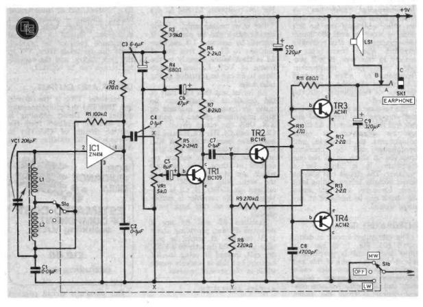
Fig. 1. The circuit diagram of the Photocube Receiver.
