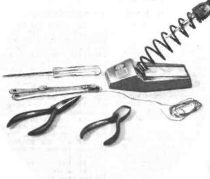
1 You will need a lightweight soldering iron with a 3 to 5mm bit, some flux cored solder and a few general tools.
