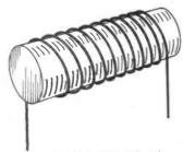
Fig. 1. A solenoid coil.
