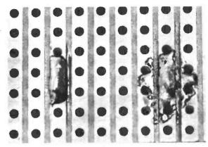
7 On the left how a good joint should look. On the right a mess made by using too much solder and keeping the iron on too long, burning off all the flux.
