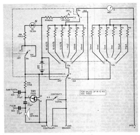
Fig. 1. The circuit diagram of the Multi-Tester.
