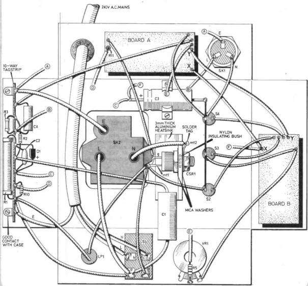
Fig. 5. Layout and wiring of the complete system.
