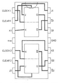
Fig. 4.2. Pin connections of the 7473 integrated circuit.
