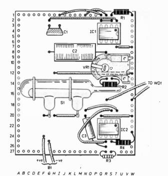
Fig. 2. The layout of the components on the Veroboard and wiring details.
