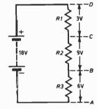
Fig. 2.3a. Shows that two points are involved when we speak of voltage.
