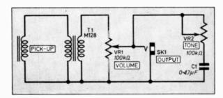
Fig. 12. The circuit diagram of the components in the control section.
