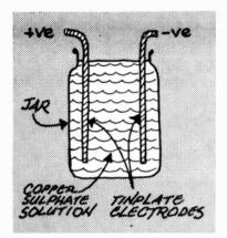
Fig. 1. Electrolysis arrangement for plating.
