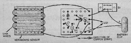
Fig. 2 The layout and wiring up details. Also shown are details for a sensor using 0.1 inch matrix Veroboard.
