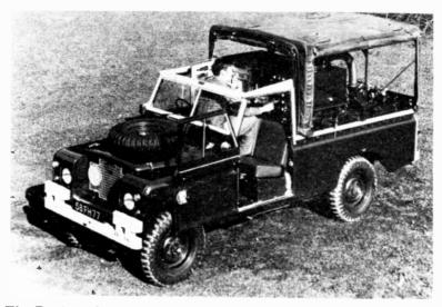
The Rapier missile forward repair and test vehicle now in service with the Army.
