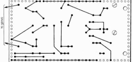
Fig. 3. Layout and wiring of the Radio Control Receiver. Readers are advised to follow this exactly.
