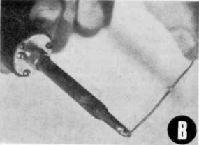
crystalised, is weak and probably has a high resistance. This could have been caused by carrying the solder to the joint on the iron, keeping the iron on the joint too long, thus burning off the flux, or by moving the wires before the solder has cooled.
