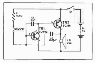
Fig. 1. The circuit diagram of the Rain/Water Alarm.
