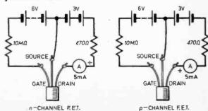
the channel is reverse biased. The greater the reverse bias, the narrower the channel width and the smaller the current which flows in the drain circuit. Connection of the gate to the 10 megohm resistor in the circuits shown will cause the drain current to fall to zero when most types of f.e.t. are being tested.
