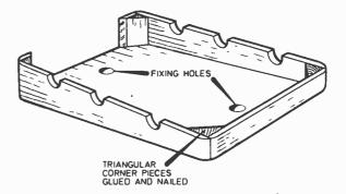
Fig. 8. Details of the head lower section.
