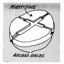
Fig. 2. The mould for making a small cross.
