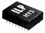
The HY5 is a complete mono hybrid preamplifier, ideally suited for both mono and stereo applications. Internally the device consists of two high quality amplifiers—the first contains frequency equalisation and gain correction, while the second caters for tone control and belance.
