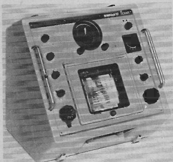
The sonar cabinet of a large fishing vessel. The dial at the top shows which way the transducer is pointing, the chart beneath presenting horizontal range to the target.
