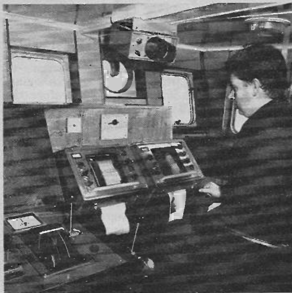
A fishing skipper studies his two echo-sounders. One is of a higher frequency than the other giving him a choice of accurate fish detection or ground discrimination.
