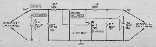
levels, the oxide layer that inevitably builds up, can act as a rectifier, setting up distortion. Three pairs of switch contacts should assist in reducing contact resistance.
