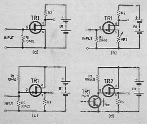
into the drain terminal and out at the source terminal (conventional current assumed). In Fig. 11.5a the gate and source are connected via a relatively high value resistor (10 megohms) but since the gate leakage current is normally very small no voltage drop occurs across R1.
