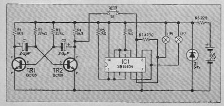
Fig. 1. Complete circuit diagram of the Heads or Tails game.
