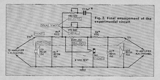
The reactance of a capacitor is, as is well known,  $1/2\pi fC$ , C being in Farads, and f in Hz. The reactance of a capacitor is inversely proportional to frequency, i.e. it is halved for every doubling of frequency. As far as this particular application is concerned, all this means is that Cl will offer a reduced resistance to the higher frequencies, so reducing the apparent sound stage for the increasing frequencies.
