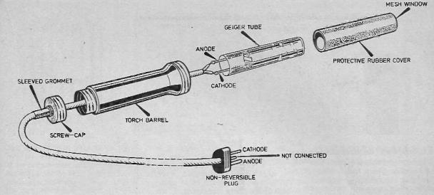
Fig. 3. Construction details for the probe.
