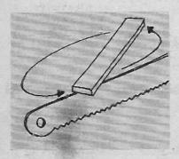
Fig. 1. Making a compass from a razor blade or hacksaw blade using a magnet.
