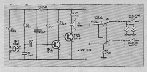
Fig. 1. Circuit diagram for the Lights-On Alert.
