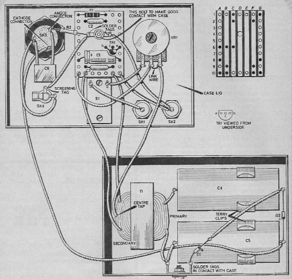
Fig. 2 (above). Assembly and wiring details within the aluminium case.
