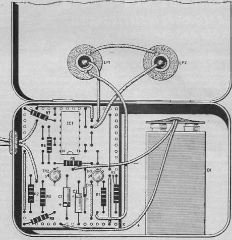
Fig. 4. Construction details of the Heads or Tails unit.
