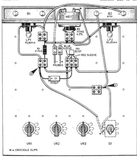
Fig. 7.5. Tutor Board layout for the circuit of Fig. 7.1. To be used with Test No. 17.
