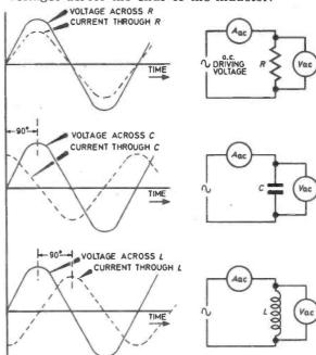
Fig. 13.1. Voltage and current relationships for resistance, capacitance and inductance.
