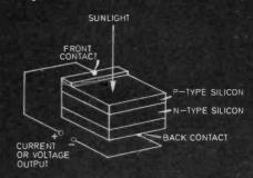
Fig. 1. Silicon solar cell.
