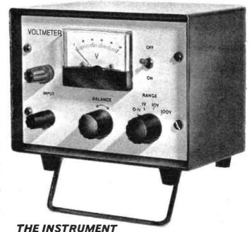
The instrument has four ranges 100mV, 1V, 10V and 100V d.c. having an input resistance 1.01 megohms. When the x10 probe is used these ranges become 1V, 10V, 100V and 1000V d.c. with an input resistance of 10 megohm. A null balance control enables the meter to be set to zero with the input terminals shorted.
