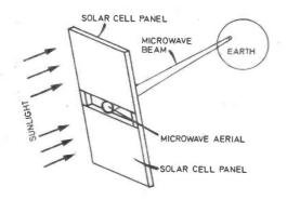
Fig. 2. Satellite solar power station. Electricity generated from sunlight is transmitted to earth at a microwave frequency.
