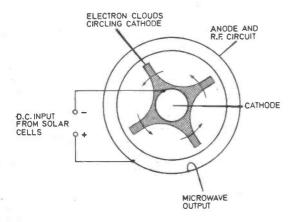
Fig. 3. Principle of operation of the magnetron valve.
