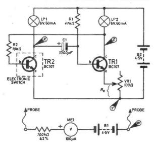
Fig. 7.4. Monostable timing circuit. The voltmeter circuit is required for test number 18.
