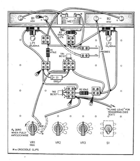
Fig. 7.6. Layout and wiring for the circuit shown in Fig. 7.4.
