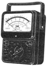
others use diodes to protect the movement against excessive current. Economies can be made by omitting this feature, but mistakes are inevitable and could lead to an expensive repair to the delicate movement.
