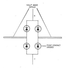
Fig. 4. Basic element of the earth receiver.
