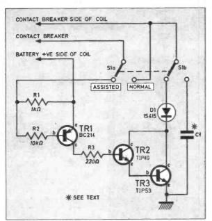
Fig. 1. The complete circuit diagram of the Transistor Assisted Ignition.
