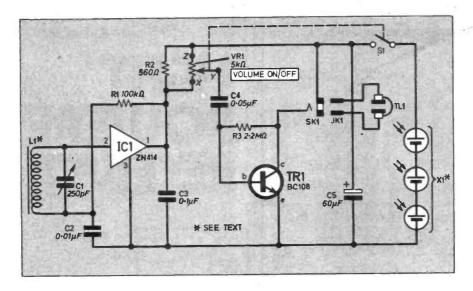
Fig. 1. The complete circuit diagram of the receiver.
