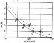
Fig. 1. Graph showing the performance of a power supply
