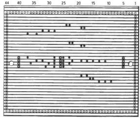
Fig. 3. Layout of the components on the topside of the veroboard and the copper regions to be removed from the underside. Note the polarity of the integrated circuit.
