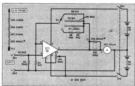
Fig. 1. The complete circuit diagram of the Electronic Voltmeter and x10 probe.
