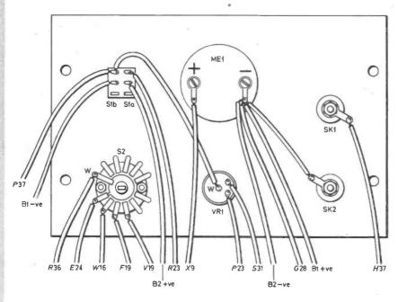
Fig. 4. Positioning and wiring up of the components on the rear of the front panel.
