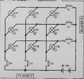
Fig. 1. Circuit diagram of the Three By Three Game.
