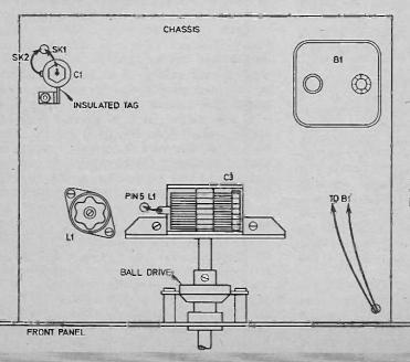
Fig. 5. Showing the positioning of the components and mounting for C3 on top of the chassis.
