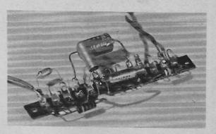
Fig. 12. Method of wiring up components on a piece of tag strip.
