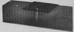
Method of mounting component board; applicable to all types of construction discussed here.
