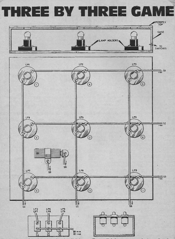
Fig. 2. Wiring of the base board and switch boxes. Two switch boxes are required, one housing S1, 2 and 3 with the other housing S4, 5 and 6.
