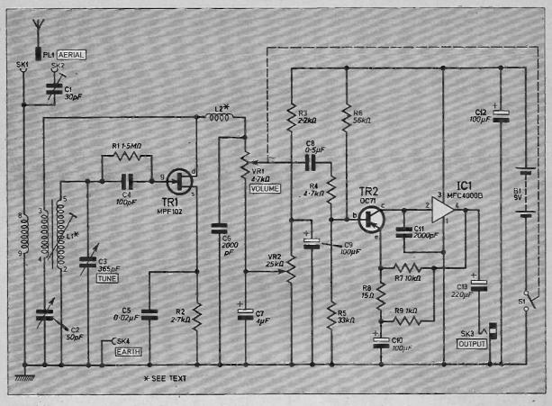
Fig. 1 Complete circuit diagram of the Four Band T.R.F. Receiver.
