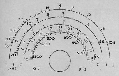
Fig. 6 Markings for the various ranges on the tuning dial this is shown full size and may be transferred directly to the scale.
