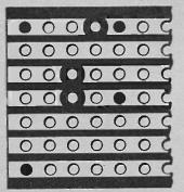
Fig. 6. Photograph and drawing of the underside of the same component board showing breaks and soldered connections.
