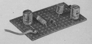
Photograph of a simple project built on copper clad Veroboard.
