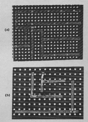
Fig. 10. Methods of placing stick-on wiring with reference to component holes.
