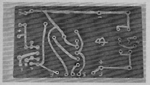
Fig. 1. The copper laminate pattern that replaces discrete wiring between components.
