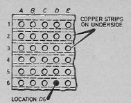
Fig. 7. Hole location using system of co-ordinates.
