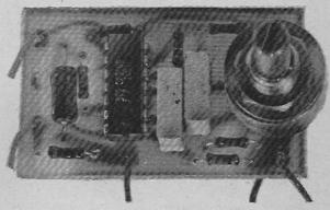
Photograph of a completed component board using the p.c. board method, illuminated from the rear.
