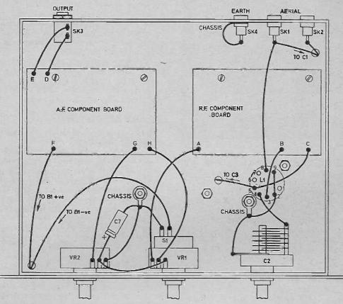
Fig. 4. Layout and wiring of parts mounted on the underside of the chassis.
