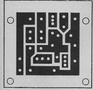
Fig. 2. The master drawing of the printed circuit.
