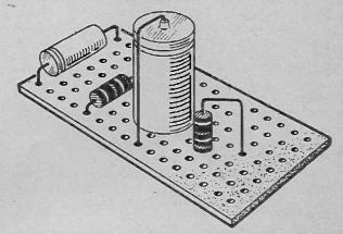
Fig. 8. Details of the two methods, horizontal and vertical, of mounting components on the component board.
