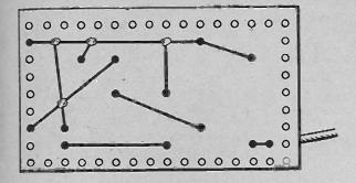
Fig. 9. Schematic of underside of component board using unclad Veroboard.
