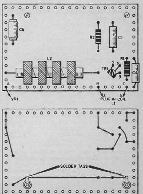
connect as shown for the underside wiring. A 20 s.w.g. tinned copper or similar wire is soldered between the tags for the metal chassis return points. In other places, the wire ends of the components are bent over and soldered as shown, and excess wire is then snipped off.
