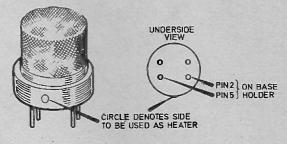
Fig. 4. Details of the sensor-
