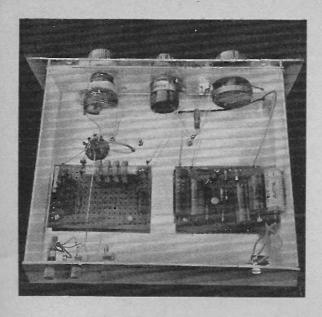
When fitting TR2, place emitter, base and collector leads in the positions e, b and c. The collector is marked by a spot on the case. The audio integrated circuit ICl has two long and two short tags, and fits as in Fig. 3. These joints should be soldered without prolonged heating and preferably a heat shunt should be clipped on the leads while soldering.
