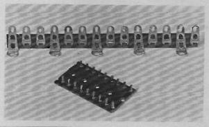
Fig. 11. A simple project wired up on a piece of standard tag board.
