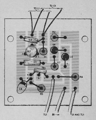
Fig. 4. Topside of printed circuit board showing component positions relative to copper pattern on underside (shown tinted).
