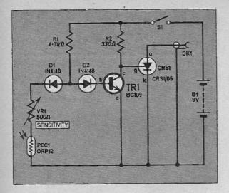
Fig. 1. The complete circuit diagram of the Slave Flash.
