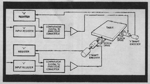
Fig. 8. Part of a numerical control system for two dimensional control-
