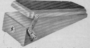
When the unit has been tested and found to work it can be dismantled and painted. It was found on the prototype that the spray on aerosol paints could easily be scratched off, so it was hand painted with a plastic enamel paint after being rubbed down and undercoated. This was found to give a very good and durable finish.
