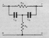
Fig. 1. A bridged-T filter used as the basis of the Waa Waa.
