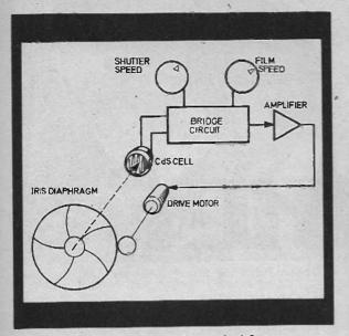
Fig. 6. Basic automatic iris control for a camera.
