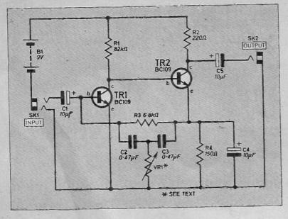
It was found experimentally that the notch position could be varied over a considerable range by varying only one component, namely  $R_b$ . Although the overall shape of the notch changes with the value of  $R_b$ , it was found to have no adverse effect on the performance for this particular application.
