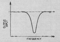
Fig. 2. Bridged-T filter characteristics.
