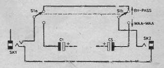
Fig. 7. Wiring details for connecting a by-pass switch.
