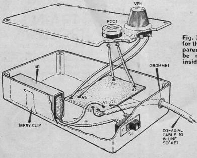
Fig. 3. The complete wiring details for the Slave Flash Unit. If a transparent case is used, PCC1 would be mounted on the Veroboard inside the case.
