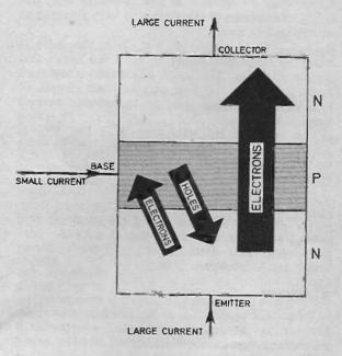
Fig. 3.9. Flow of charge carriers in the npn transistor.
