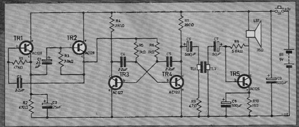
Fig 1. Circuit diagram of the Electronic Doorbell.
