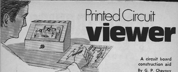
CHECKING a printed circuit board, or tracing a circuit off a printed circuit board can be a tedious and time-consuming task. However, by using the Printed Circuit Viewer described here, the job is made so much easier as it is possible to see the components on the top of the board and the copper circuitry underneath the board, at the same time.
