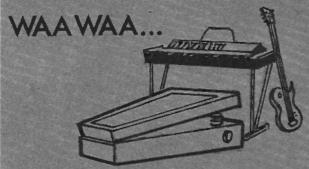
For use with guitars, organs etc. This effects unit has been designed to be easy to build and uses no inductors.
