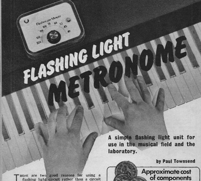
THERE are two good reasons for using a flashing light circuit rather than a circuit that generates an audible tone, firstly, an audible signal gets lost amongst amplified music, and secondly, a flashing light is less annoying than a continuous clicking sound.
