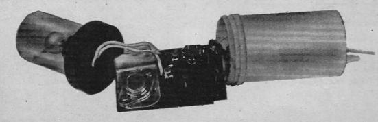
The complete unit could be self contained within a commercial plastic dome lamp together with a battery and control switch. Finally the unit may be constructed complete, as in the prototype, housed in the case design shown in the photographs and diagrams.
