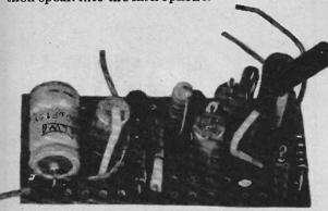
The Veroboard housing the amplifier used in the Intercom.
