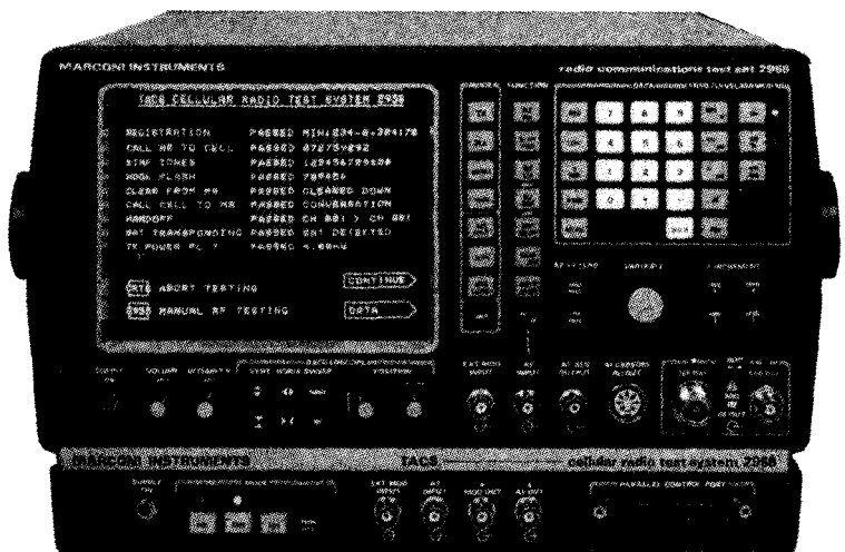
A cellular radio test set. An adaptor, the Marconi 2958 talks to the Marconi 2955 via GPIB
