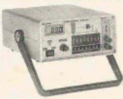
Instrumento preciso e prático, nas escalas de 200 pF, 2nF, 20 nF, 200 nF, 2  $\mu$ F, 20  $\mu$ F, 200  $\mu$ F, 2000  $\mu$ F, 20 mF.
