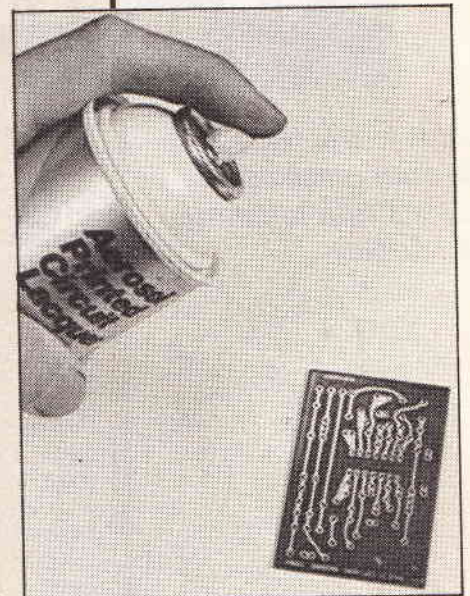
Protecting the circuitry with a lacquer
