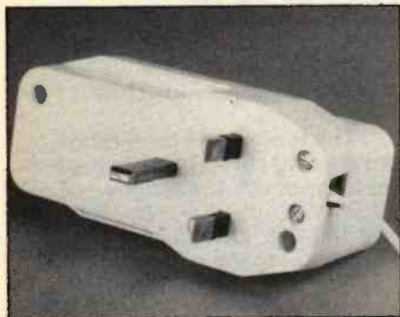
The mains transformer module.
