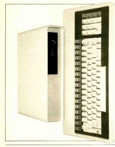
keyboard and 3.5" disc drive. Details of this and other case options will be The 6809-based microcomputer fitted in a Vero case and equipped with a given next month.
