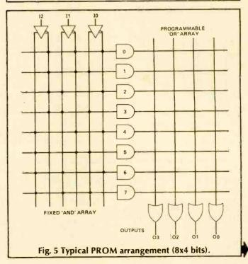
PROMs have the advantage of low cost and are relatively easy to program. However, since the AND array is fixed, with one gate for each combination of inputs the chip size increases rapidly with the number of inputs. In fact, the total number of AND gates will be equal to 2 raised to the power of the number of inputs. For example, a 16-input PROM will have 64,000 locations. In the vast majority of applications such a PROM would be heavily under utilised.
