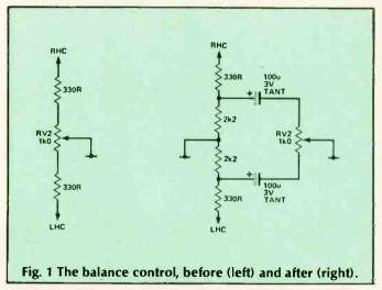
6. The balance control carries DC current intentionally to ensure that constant resistance is overcome. This does mean that there is an audible brushing noise whenever the control is turned. If this proves an irritation the circuit modification shown in Fig. 1 can be made. The balance control must be a wirewound type. Any other type will degrade the stereo separation. In my opinion, this modification worsens the sound quality.
