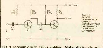
Fig. 9 Economic high gain amplifier. (Note: all circuits use general purpose silicon transistors operating at lower power AF or RF frequencies).
