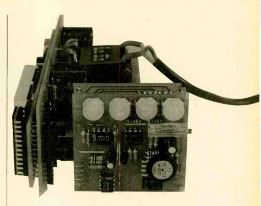
links line up with the holes on the motherboard. When this has been done, the module can be fitted onto the motherboard and soldered. Trim off any excess from the links. Alternatively, you can use SIL PCB sockets on the motherboard and just push the bent links into them.
