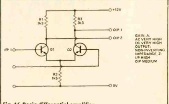
Fig. 16 Basic differential amplifier.
