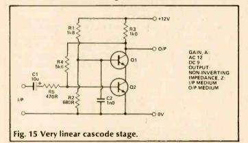
The configuration is widely accepted as a very high frequency amplifier displaying extremely good linearity. This feature is useful for quality audio, and the circuit can often be found in amplifier systems.
