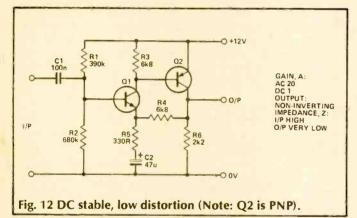
Distortion tends to increase with gain, but can be kept down by the use of complementary transistors (the BC182/BC212 pair would be suitable here). As with the Fig. 10 circuit above, frequency response can be tailored to the user's requirements by including reactive networks in the feedback loop. If the gain is lowered too much at HF, circuit stability might suffer with spurious oscillations as the result.
