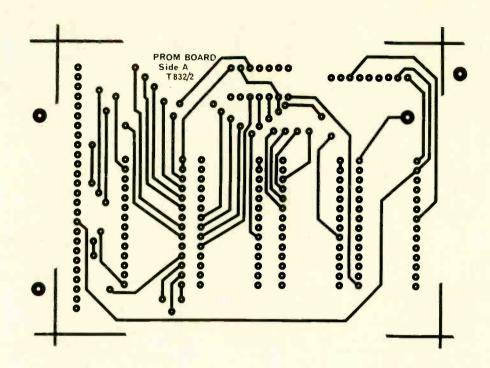
The top and bottom foils for the 6809-based microcomputer EPROM disc board. The foils for the main board are too big to reproduce here but made-up boards are available from Micro Concepts. See the Buylines section in the article.
