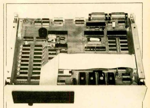
Another view of the cased board. Note that the EPROM disc board shown here (lower centre-right) is a prototype.
