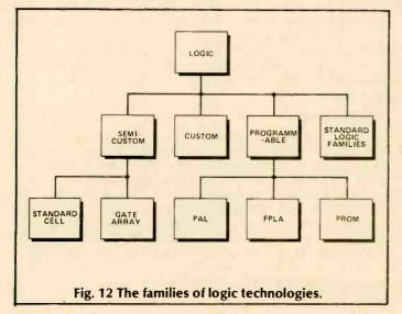
The designer of both standard cell or gate array devices is faced with almost indistinguishable development tools, the differences which are transparent being of relevance only at the manufacturing stage. From a customer point of view the only difference is in the pricevolume relationship. Performance and interfacing requirements are very similar.
