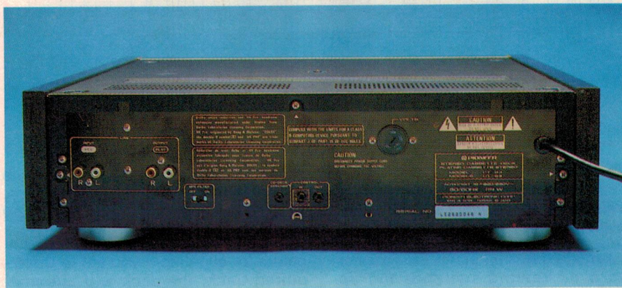
Along with the usual stereo in and out connectors, the Pioneer CT-93 rear panel has a multiplex filter switch, sockets for remote control and a further socket for the CD deck synchronisation feature.
