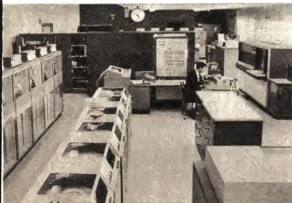
The original IBM System/360 Model 50 installed at the IBM data centre in St. Kilda.
