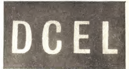
Simple DCEL letter display, photographed from its own illumination. The letters can be obtained either by evaporating the back electrode through a mask, or, as in the example illustrated, by photo-etching the transparent electrode.
