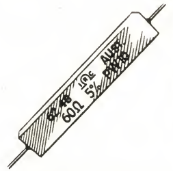
4. Ceramic case Wire wound Fireproof inorganic construction 5 to 15 watts.
