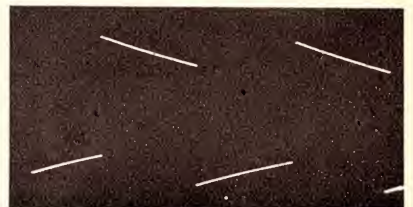
Excellent low frequency power response is indicated by the above square wave response measured at 100Hz with a power level of 40 watts.
