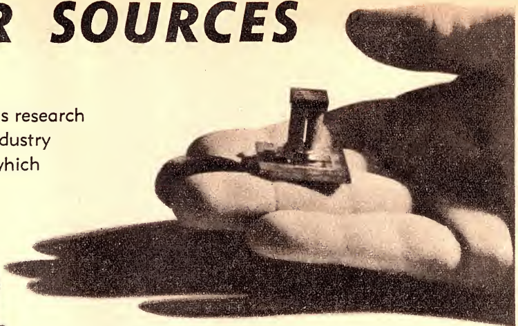
Germanium-silicon thermocouples, which convert heat to electricity.
