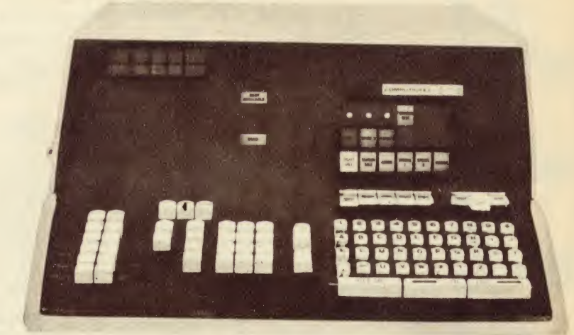
The terminal unit of the "Computicket" machine. Once the operator punches in the request, the response of the machine is almost instantaneous. The machine also prints the tickets.
