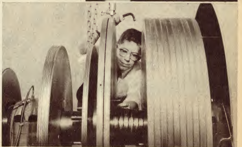
BOTTOM: Part of the massive dynamometer used for testing brakes. Vehicles of different weights can be simulated by selection of appropriate discs.
