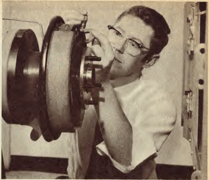
TOP: Measuring the thickness of brake linings during dynamometer tests on a braking system.
