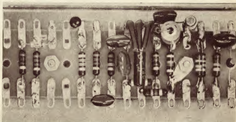
This photograph of the "signal path" board should be studied and correlated with the wiring diagram shown on page 81. The emitter-follower stage is at the right, with the gating transistor next and followed by the amplifier and switching diodes at the left.
