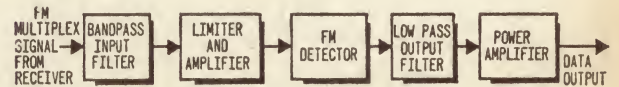
Figure 7. Block diagram of a typical subcarrier discriminator. First block, bandpass input filter, selects a very narrow range of frequencies that is related to a specific telemetry channel.
