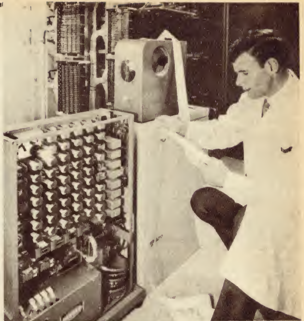
The PETRA Call Analyser undergoing field trials by the Post Office in Melbourne. The tape printer is standing in its normal operating position, on top of the cover, which has been removed to show the interior of the equipment.
