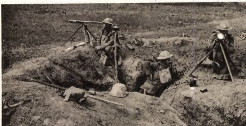
During World War I the heliograph was widely used for sending messages over short distances. In this picture, the device is being used for transmitting messages back from a forward spotting position to an artillery post.
