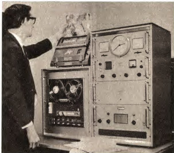
This A.P.T. receiving system, installed at the British Meteorological Office, is similar to the ones to be supplied to the New Zealand D.C.A.
