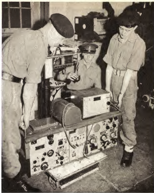
A British Army No. 52 set for telephony, CW and MCW, in use at the time of the Suez crisis and the Korean war.
