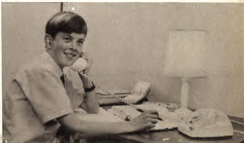
In external appearance, the telephone set developed for the use of deaf persons differs little from the normal set. Note, however, the potentiometer control to the lower right of the dial.
