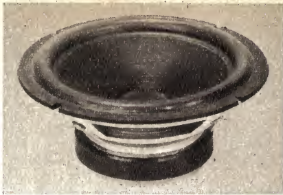
A typical, modern 6-inch low frequency drive unit, as produced by Rola. Because of its reduced cone area, it can be used in a smaller enclosure than, say, a 12-inch unit.
