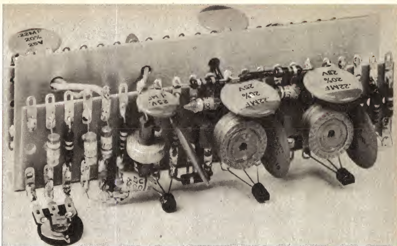
IF amplifiers, following the filter assembly, with input at right and the AM-SSB detector at the left. Note the balancing potentiometer.
