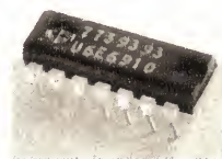
An enlarged photograph of the integrated circuit is shown above. It is a 14-lead dual in-line package with a locating slot at the right hand end.
