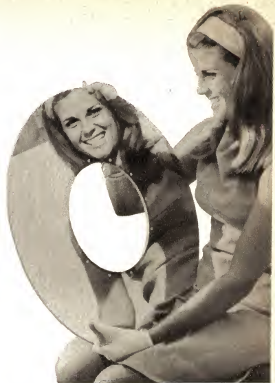
The 16in disc used in the recorder. The high quality of the polished surface is indicated by the perfection of the reflected image.
