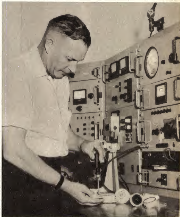
P.M.G. research technical officer Jack Laughlin fits the external hearing aid coil for the telephone developed specially for the use of deaf persons.
