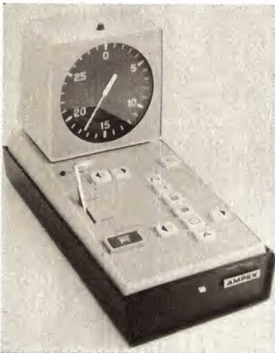
The control unit showing control buttons and cueing clock. It includes a fast search facility which can locate any part of the recording in four seconds.
