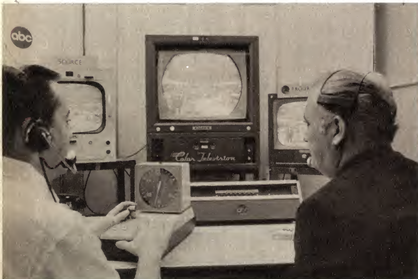
A typical control position setup for a sporting event, showing the video disc control unit with cueing clock. This unit provides all the control and cueing facilities necessary to operate the recorder.
