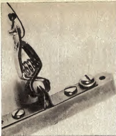
A simple foot trap unit. The circuit between the two pieces of brass is normally completed by the alligator clip, to which is attached the trip thread.
