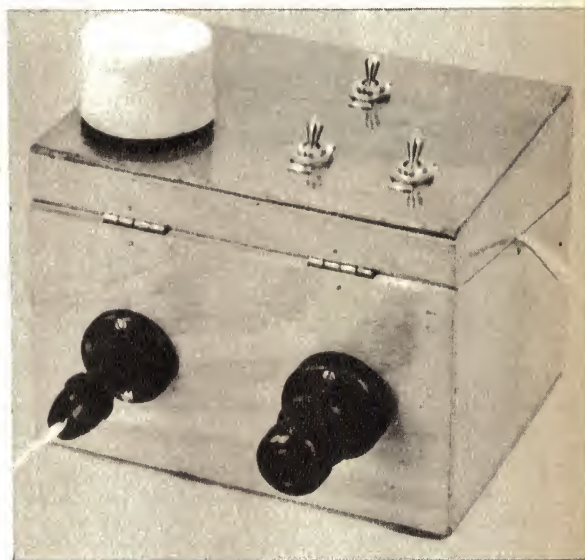
The control unit is built in a wooden filing card box. On the lid is the master switch, a switch each for the bell and buzzer, and the buzzer. The two sockets serve the bell and window contacts respectively, while the flex at the right is for the battery.
