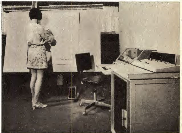
An operator guides the reading head across a map while using the Gerber Digitiser.
