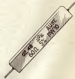
4. Ceramic case Wire wound Fireproof inorganic construction 5 to 15 watts.
