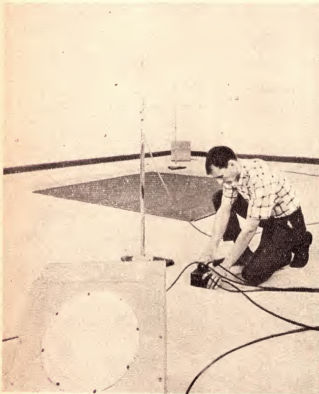
LEFT: Setting up an experiment for measuring the sound absorption properties of a rug in the reverberation chamber.
