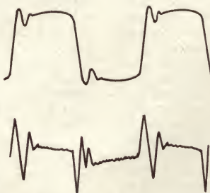
Traced from the oscilloscope screen, these are transient patterns obtained with a typical high quality magnetic cartridge. At the top is the intended square wave produced by normal replay conditions with RIAA equalisation. Below it is the pattern produced under constant velocity conditions, and no equalisation.
