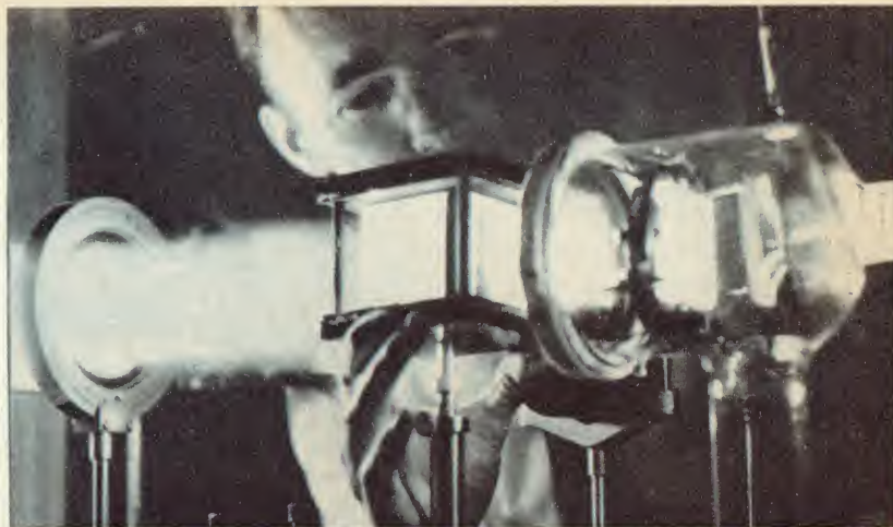
Experimental set-up for producing images on photochromic surfaces by exposing them to light of one colour through a negative, and erasing the image by light of another colour.
