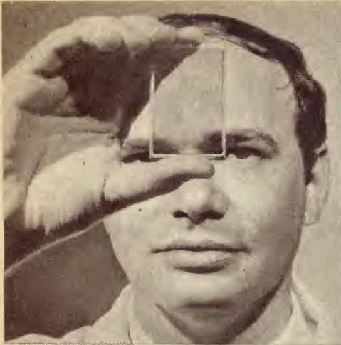
Portrait image obtained on a photochromic surface by exposing it to blue light through a photographic negative. It can be erased by exposure to yellow light.
