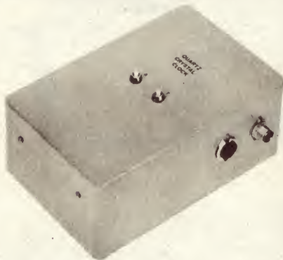
Another view of the complete unit, showing the DC power input socket (two-pin) and the 50Hz output socket (coaxial).
