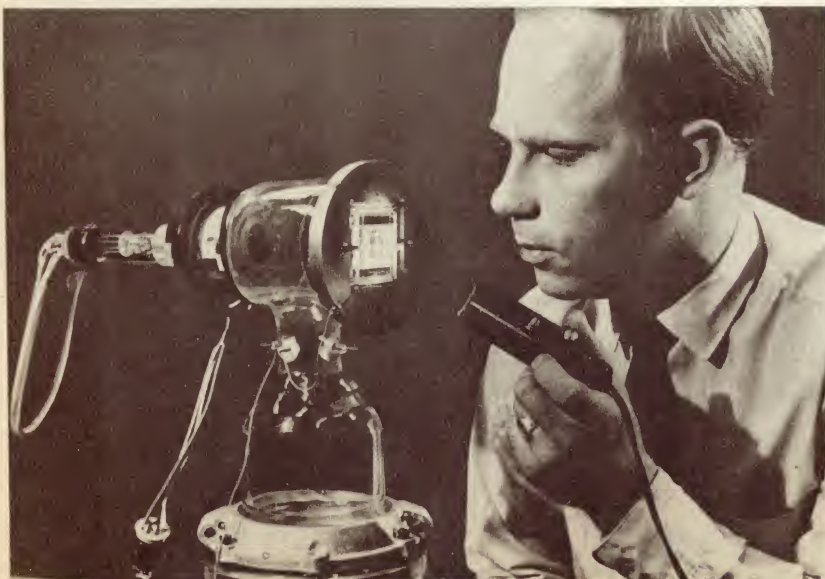
A TV test pattern from a New York station received at the RCA Laboratories is displayed on a liquid crystal screen.
