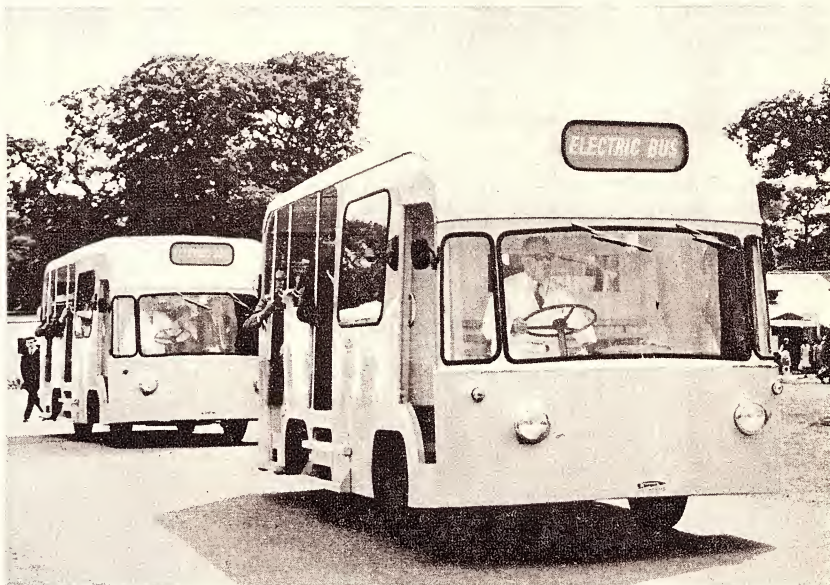
Experimental battery-operated electric buses with seating for 29 passengers, developed in the U.K. by Austin Crompton Parkinson. Powered by a fuel cell/battery combination, these vehicles would have longer range and could compare favourably with diesel powered vehicles in running costs.
