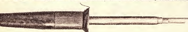
M150 Tip Shaft Dia: 5/16" Rating: 45 watts Weight: 6 ozs. Application: General Purpose Solder Tool, sheet metal, earthing strips and other heavy duty work. Tip incorporates unique anti-seizing ferrule
