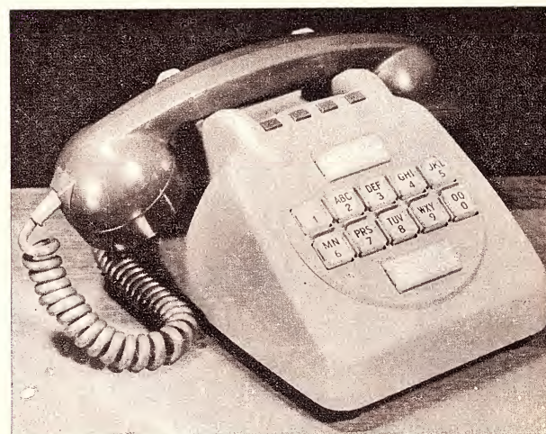
One of the push-button dialing handsets. Adjacent to the hand-piece are four auxiliary service push buttons offering additional facilities.
