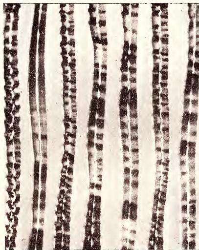
Figure 6: A much enlarged photograph of a stereo recording, reproduced by courtesy of Cecil E. Watts. Note the difference between the modulations on the respective groove walls. The average groove width is also seen to vary as signal components resultants have produced vertical modulation and either raised the cutter tip or forced it more deeply into the surface.
