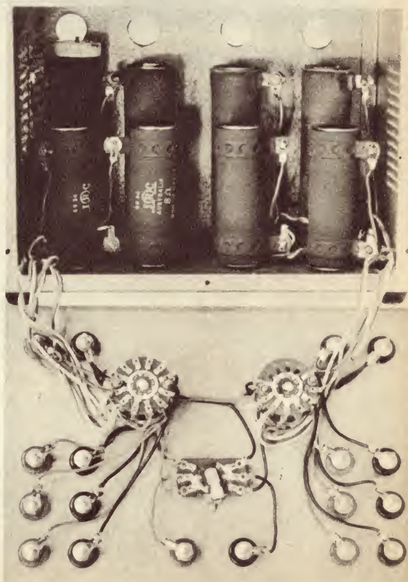
Above: The complete unit built in a standard instrument case. Right: Rear view showing resistor mounting and switch and wire layout.
