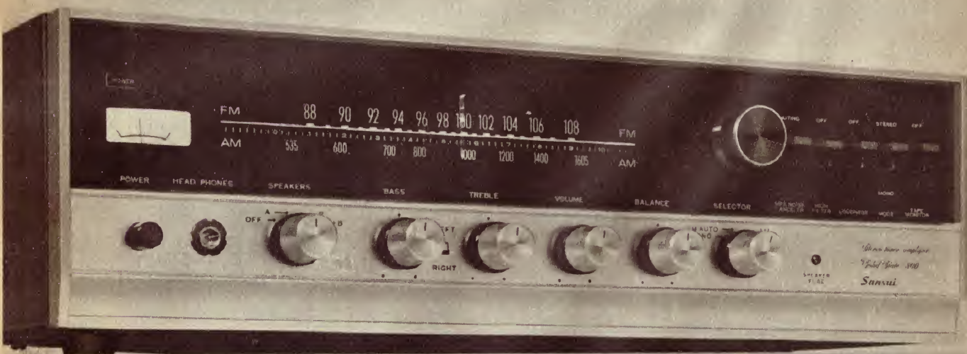
Sansui 800 Solid State AM/FM Multiplex Stereo Tuner Amplifier. 70 watts. FET & IC circuitry. Bandwidth: 20 to 35,000Hz. Distortion: less than 0.8%.
