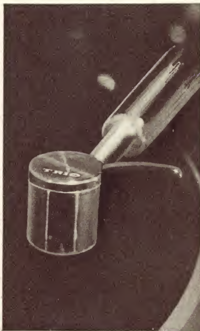
The Trio Supreme 20 cartridge is encased in an integral head shell as illustrated.
