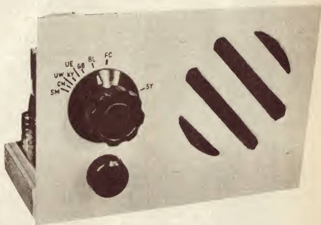
Front view of the "Micro-Plus" version of the receiver, which drives a loudspeaker. At left is the new LM372 microcircuit, approximately actual size.
