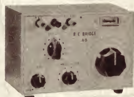
R.C. BRIDGE (MAY, '66)
