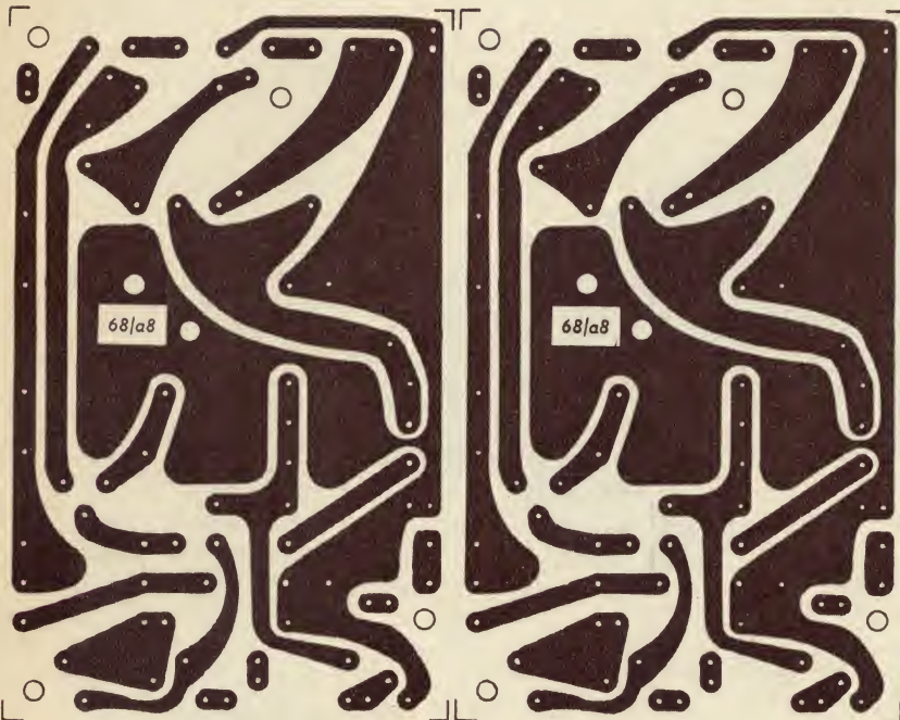
Above is the copper pattern of the amplifier board. Actual size of the board is 5\frac{1}{2} \times 4\frac{1}{2} inches.
