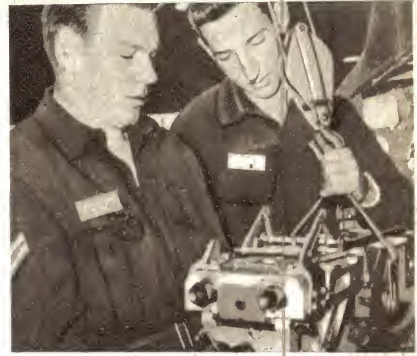
Armament. Armament Fitters fitting a 30 mm. Aden Cannon to a mock-up of a Sabre fighter.
