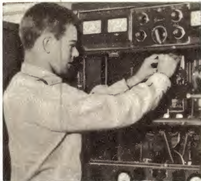
Radio. Radio Technicians (Ground) adjusting 3-Kilowatt high-frequency transmitter.
