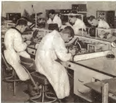
Instruments. Instrument Fitters reconditioning aircraft gyroscopic equipment at No. 2 Aircraft Depot, Richmond, N.S.W.
