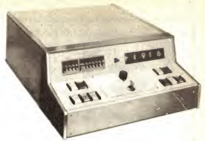
All manual controls of the Solartron IDAS system are contained in this compact desk top unit.
