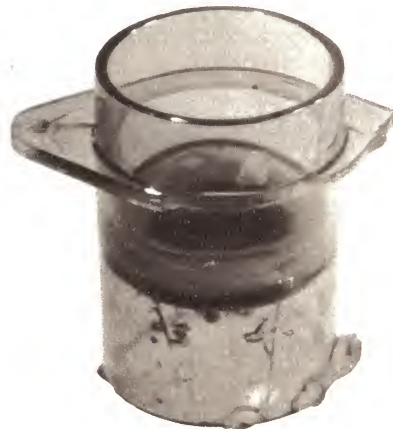
Heavy-handed assembly in the factory had caused this EHT rectifier socket to crack, providing an air path for arcs to the "outside world".
