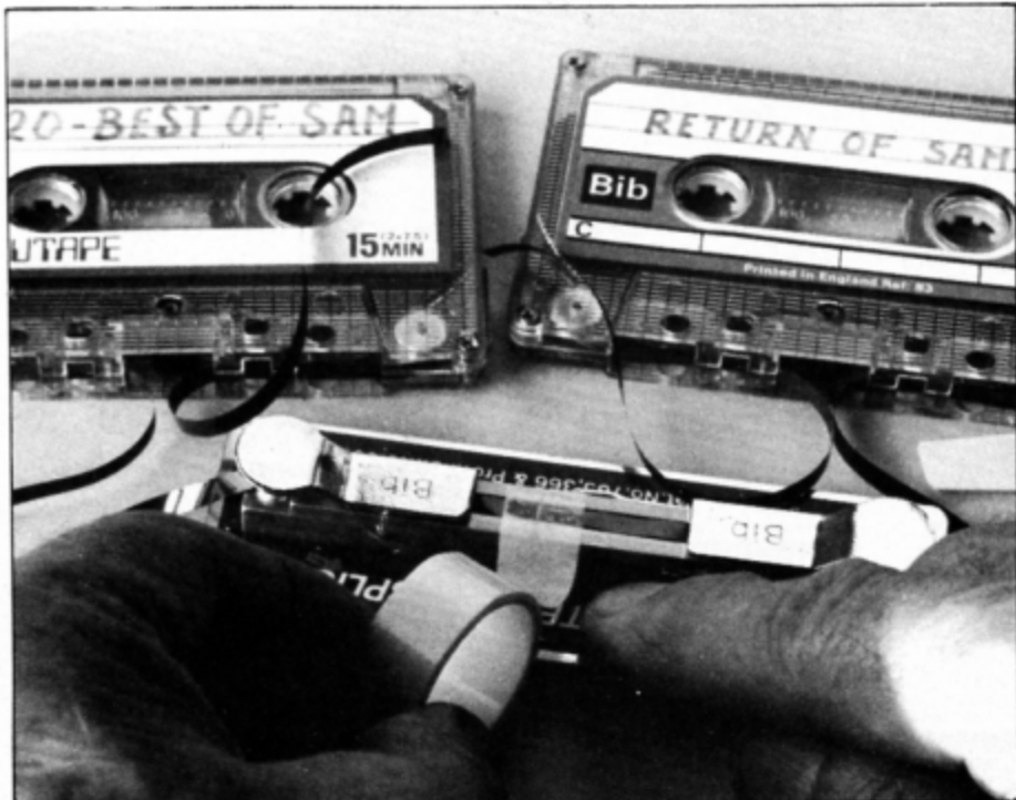
Tape from the left spool is joined to the right spool of the new cassette
