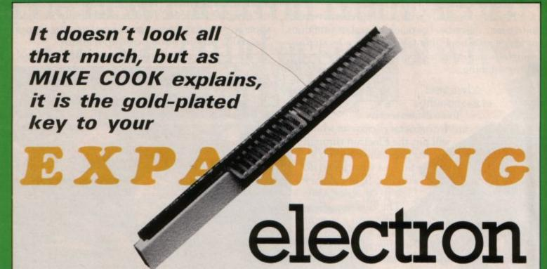
HIDING at the back of the Electron, covered by a slip-on plastic protector, is a double sided, gold plated, 50-way edge connector.
