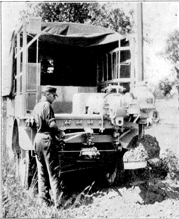
Figure 5—Boring Mechanism and Control Levers with Auger Rack in Vertical position
