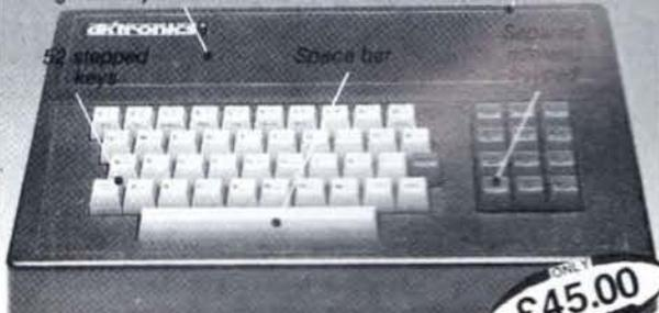
numeric data entry. The 15" x 9" x 3" case will accommodate your Spectrum and other add-ons like interface 1, power supply etc. and forms an attractive self-contained unit. All connections, power, Mic, Ear, T.V., network, RS232 and expansion port are accessible at the rear. A few minutes, a screwdriver and the simple instructions supplied are all you need to fit your Spectrum. All **tronics** products are covered by a comprehensive guarantee.
