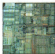
The L2 cache is a 256K SRAM package on the same chip as the CPU. The CPU has 5.5 million transistors, but the cache requires 52.5 million to avoid refreshing every 70ns
