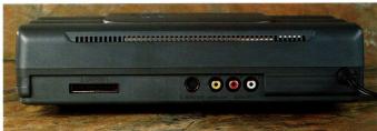
The rear of the Sanyo TRY machine is clean, uncluttered and much the same as all the other 3DO models. Left to right: expansion port, S-VHS port, composite video port, audio (left and right) ports, power supply cable.
