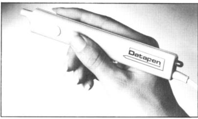
Datapen's light-pen - with LED readout and built-in switch
