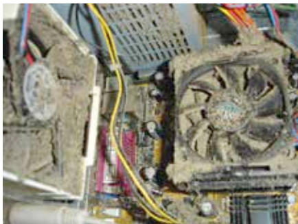
Dust clogs up on the fans and makes them noisy
