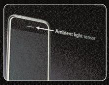
The iPhone's inbuilt Ambient Light Sensor automatically adjusts the display's brightness in accordance with the ambient light
