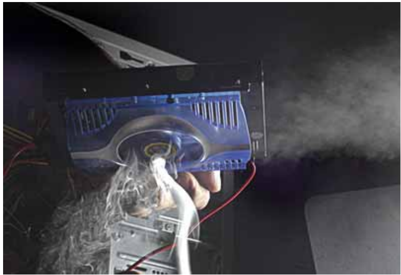
The hard disk cooler sucks in air from below and is supposed to blow it out both open sides, but for some reason, it would do so out of only one side. Go figure.
