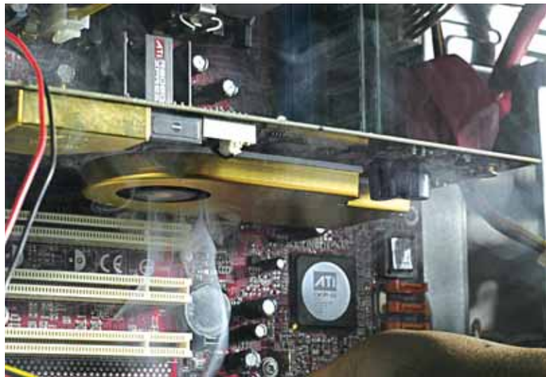
This X1300 graphics card blew air into the most inconvenient place possible—when buying, please make sure that your card's heatsink blows out of your cabinet!
