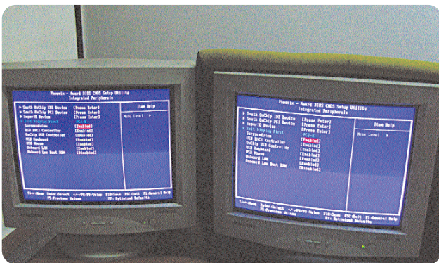
The BIOS and Startup screens are displayed on the two monitors connected to the GPU. The onboard is enabled after Windows starts
