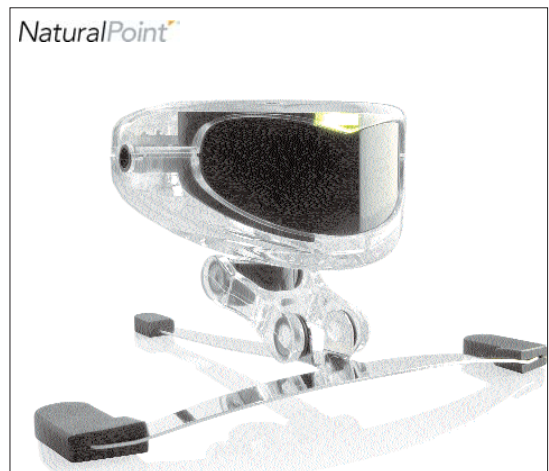
TrackIR 4 Pro translates head movements into mouse movements on your screen
