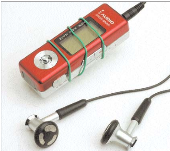
Wrap a wire around for better FM reception indoors
