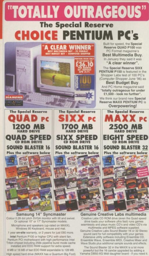
High speed hard drive (MAXX has a Quantum Big Foot) & 1.44 MB floppy drive. Enhanced IDE, 7 drive bays, 3 32 bit PCI slots and 4 16 bit ISA slots.
