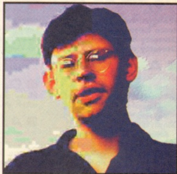
▲ The left half of the image has been saved with JPEG quality set to minimum, the right half with quality set to maximum. The left-hand side file takes up 2,800 bytes, the right side takes over 65,000 bytes. JPEG is a constant struggle to find a balance between file size and quality.
