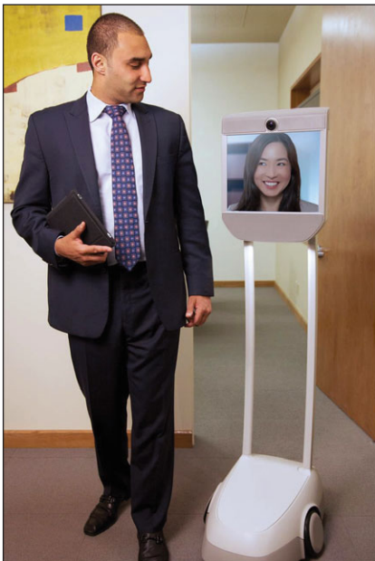
One selling point of tele-robots such as this Beam model from Suitable Technologies is that their mobility enables remote workers to communicate with co-workers beyond the constraints of traditional videoconferencing.
